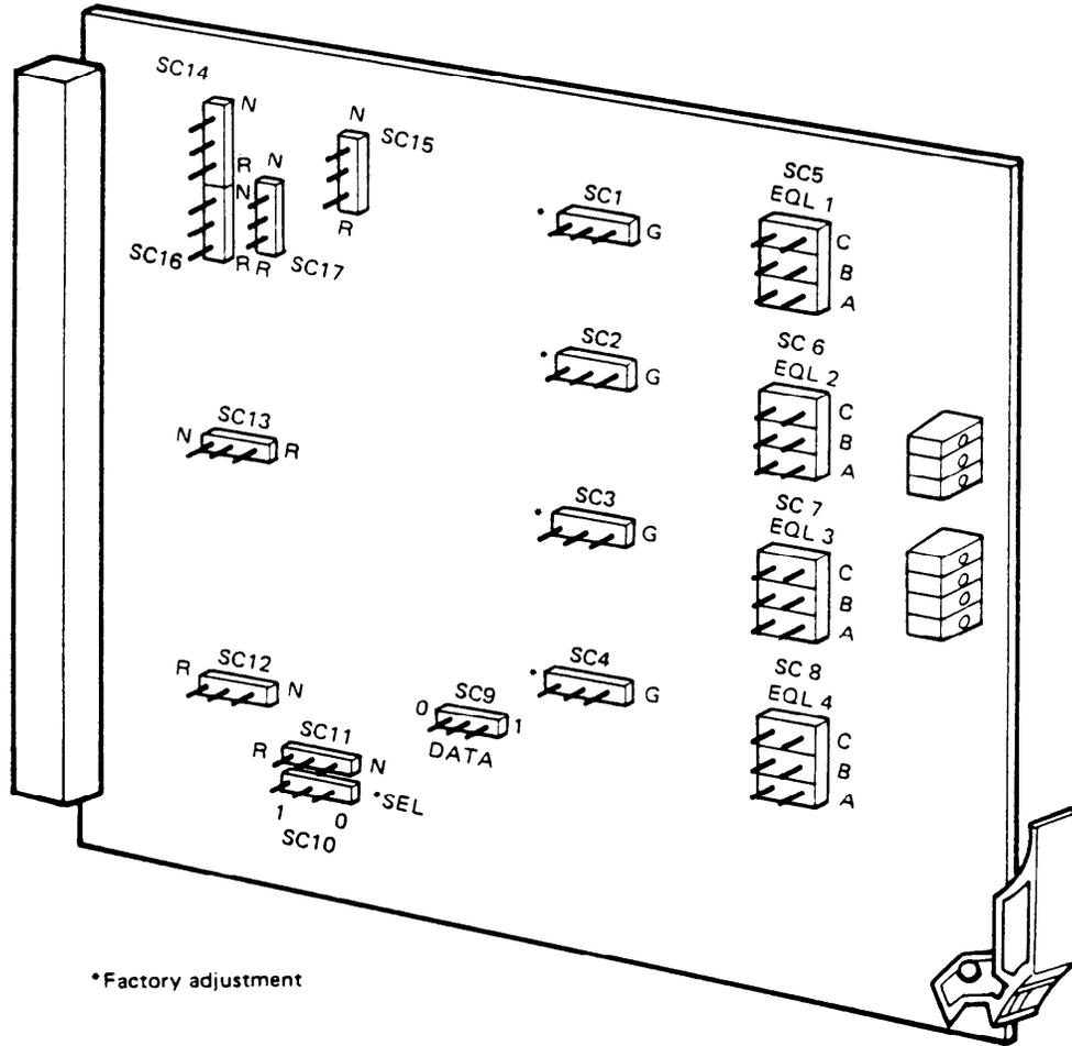
◆ Figure 5-7 DMUX Unit (Grp: 0A01/0B00) Straps Location (Sheet 1 of 2) ◆
