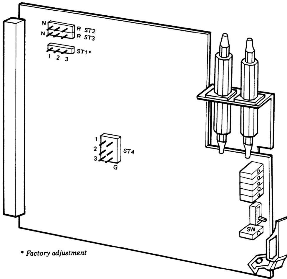
Figure 5-13 6M OPT INF (X0307) Unit (Grp: 0C01, 0B00) Straps Location (Sheet 1 of 2)
