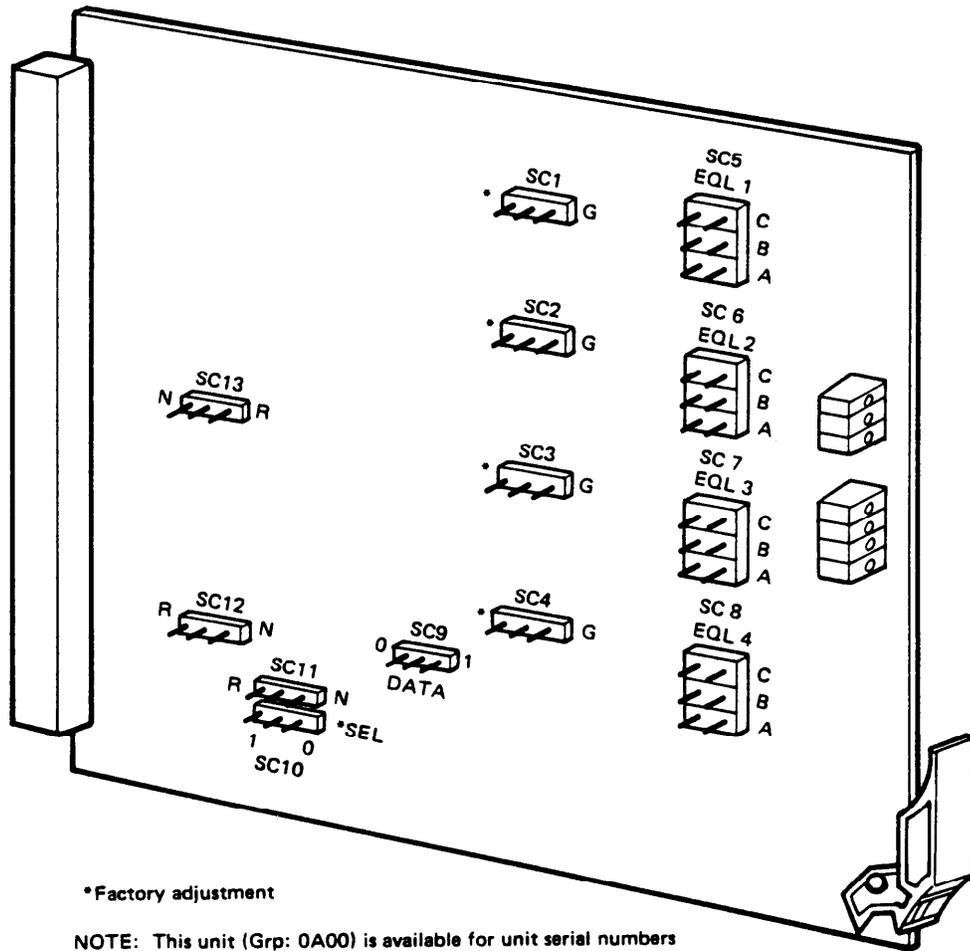
Figure 5-6 DMUX Unit (Grp.: 0A00) Straps Location (Sheet 1 of 2)
