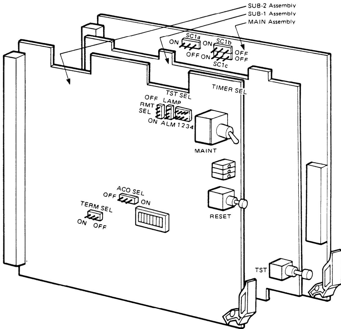
◆ Figure 5-3 ALM Unit (Grp: AA00/AB00) Straps Location (Sheet 1 of 2) ◆
