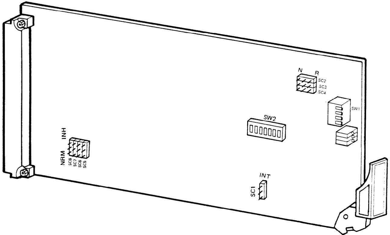
◆ Fig. 5-10A MUX Unit (GRP: 0A02/0B02) Options Location ◆
