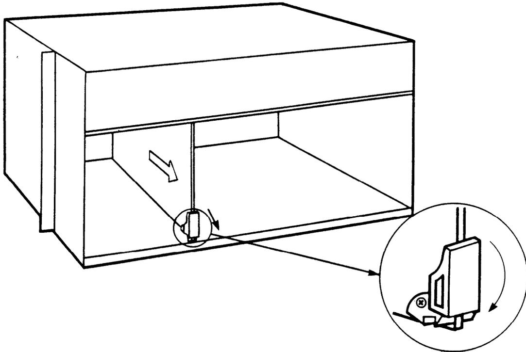
1. When the ejector is pulled down, the unit is disconnected from the connector at back of shelf.
