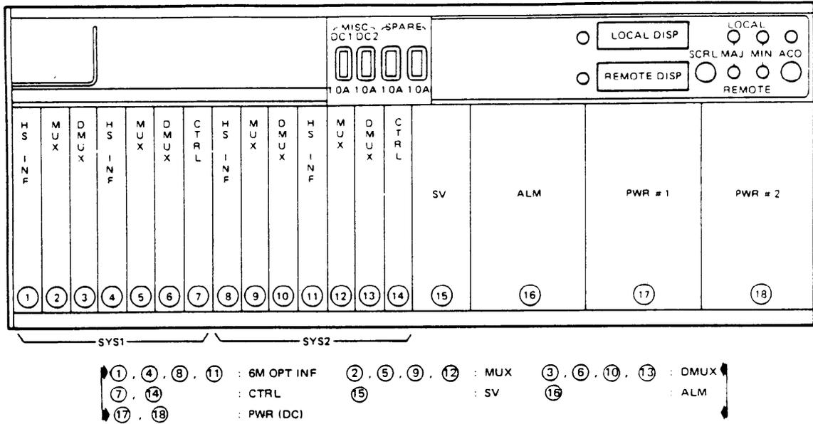
(A) Optical Interface of Redundant Configuration for DC Application
