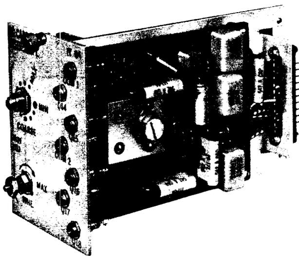
Fig. 4—Old Model Supergroup Carrier Distribution Amplifier Module Having COARSE and FINE GAIN ADJ Controls
