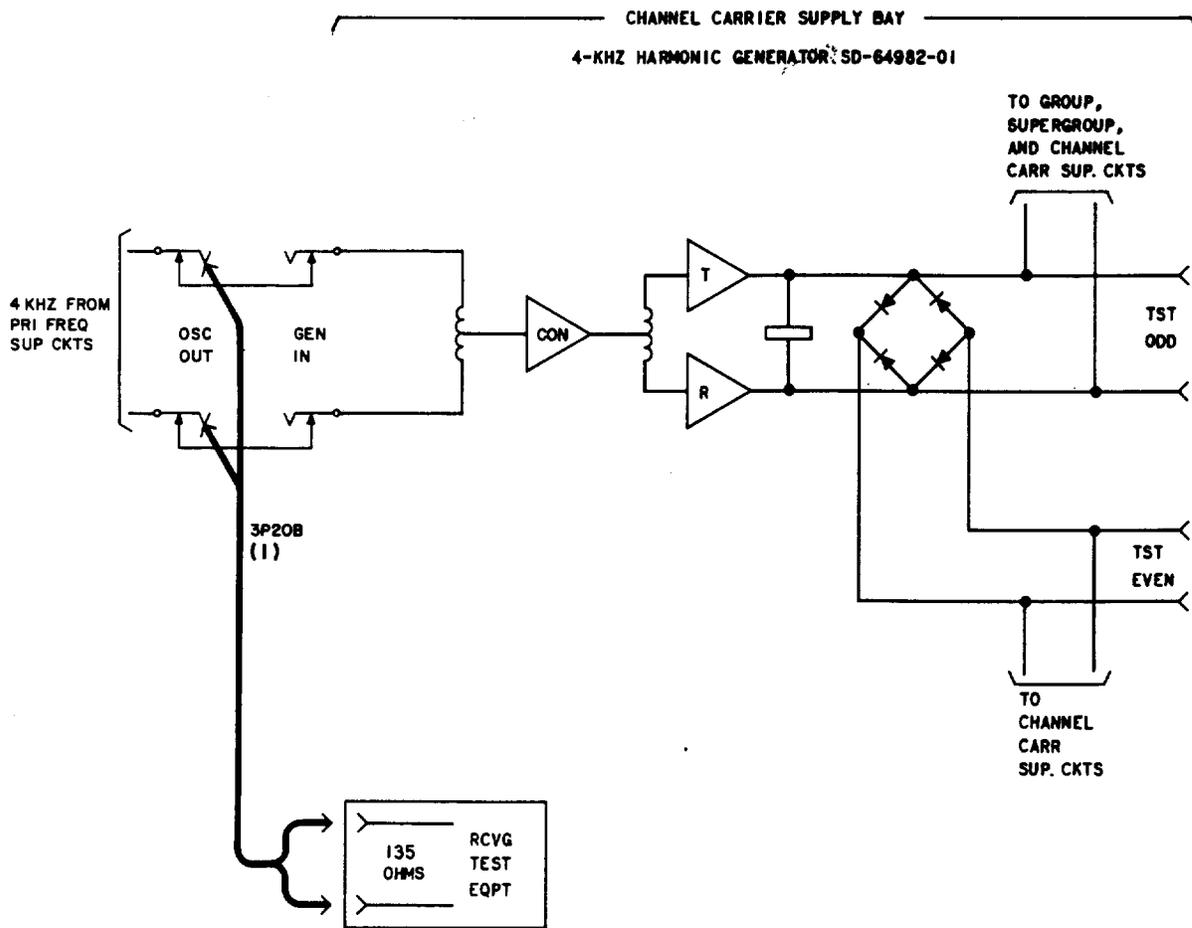
Fig. 1—Channel Carrier Supply Bay—Measurement of 4-kHz Output Power From Primary Frequency Supply
