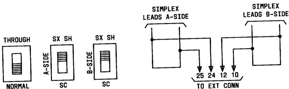
Fig. 13—Switch Settings for SD Repeater to Furnish a Sealing Current Sink
