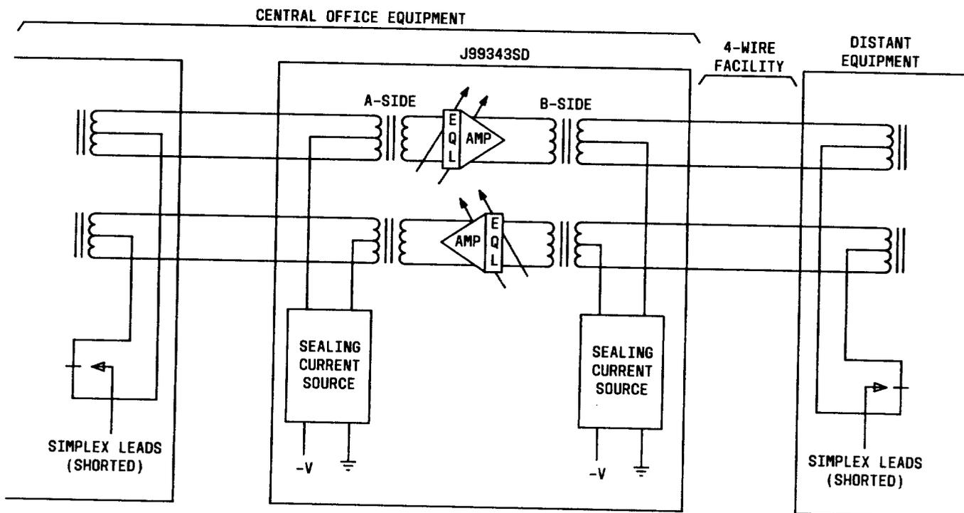
Fig. 17—Typical Application of the J99343SD 4-4 Wire Repeater With Sealing Current
