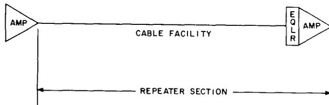
**Fig. 3—Repeater Section**
