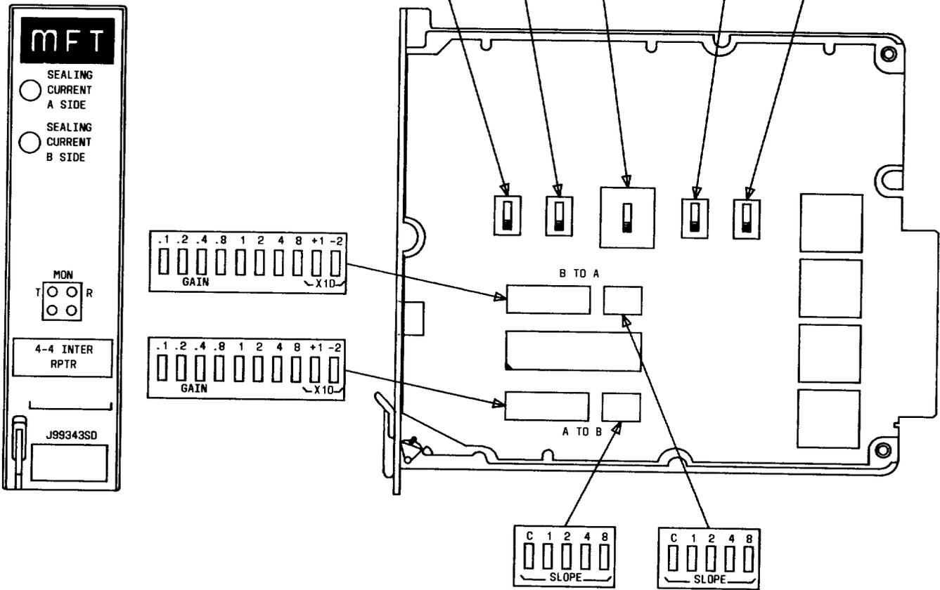
Fig. 2—J99343SD 4-4 Wire Repeater—Switch Layout
