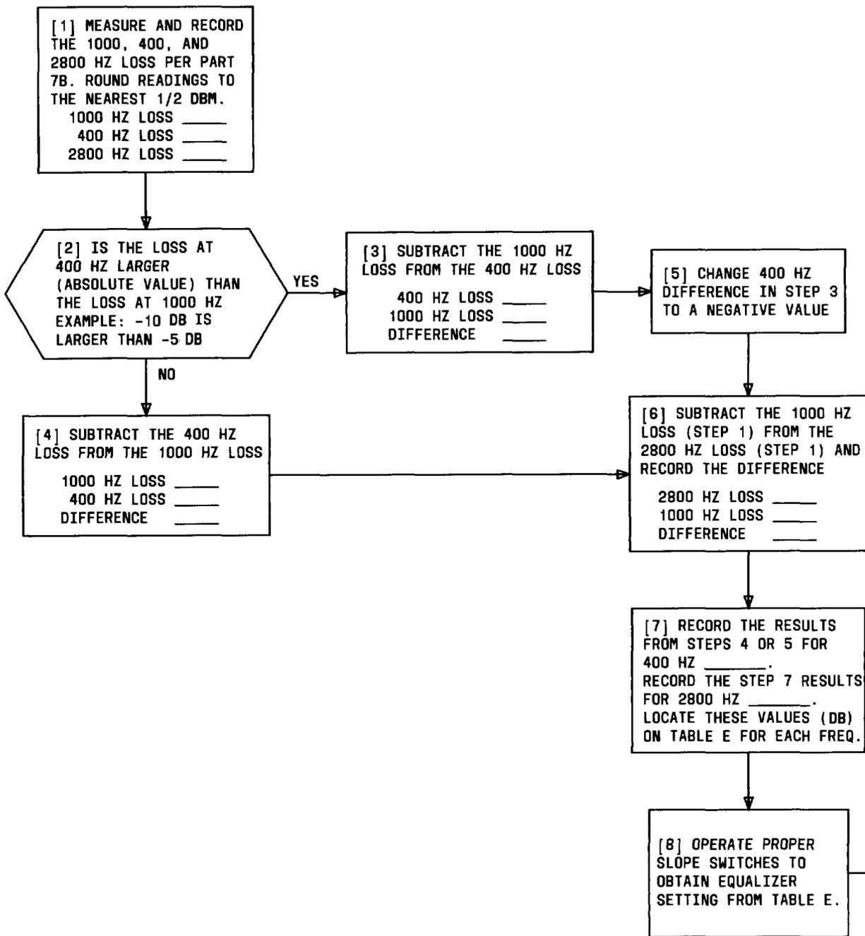
Fig. 9—Obtaining Equalizer Setting By Measurement
