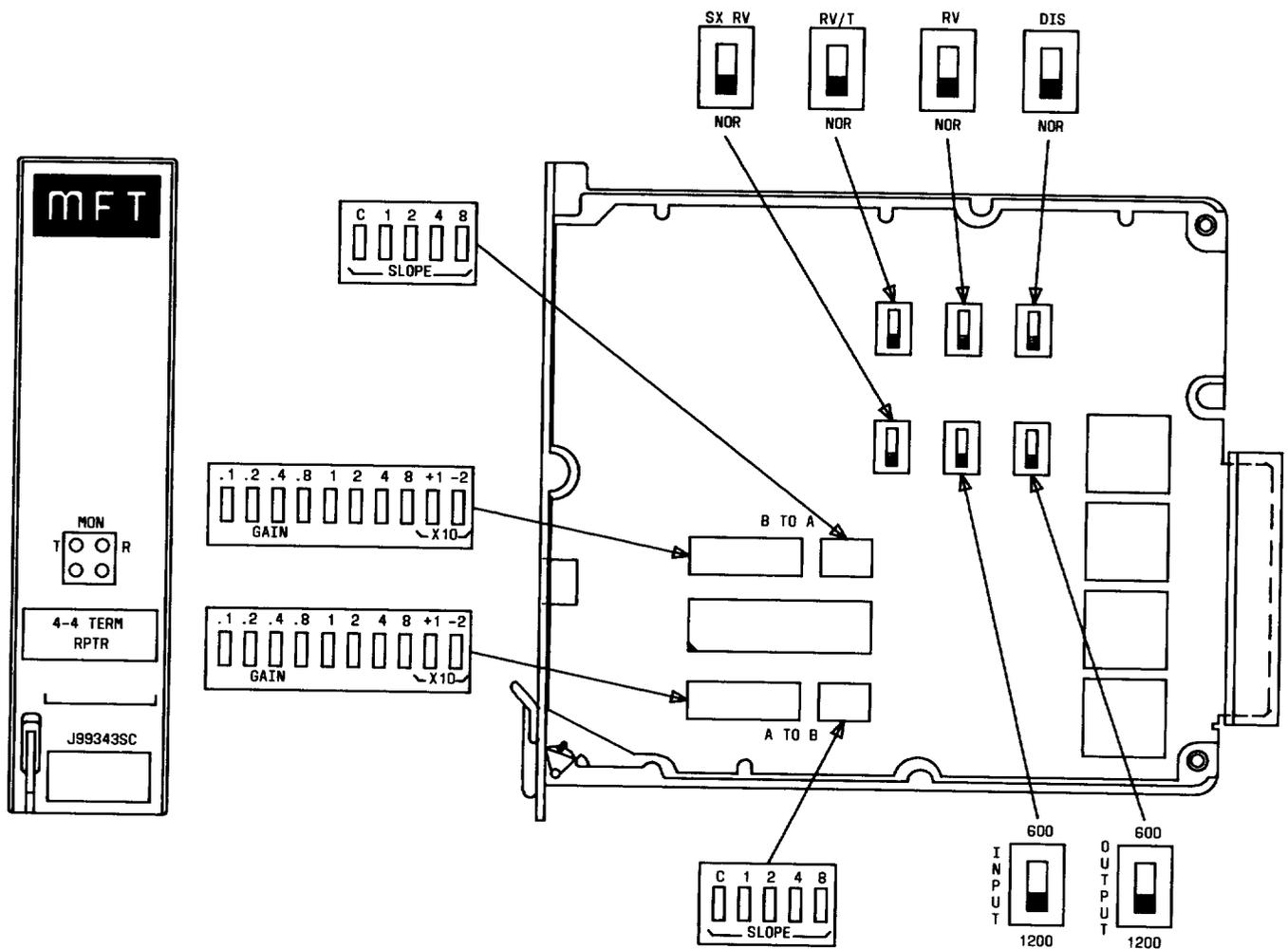
Fig. 1—J99343SC 4-4 Wire Repeater—Switch Layout
