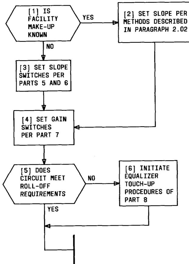
Fig. 4—Transmission Alignment Sequence
