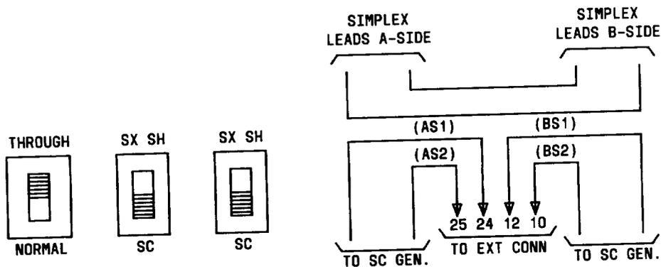
Fig. 12—Switch Settings for SD Repeater to Furnish a Sealing Current to External Circuits Only
