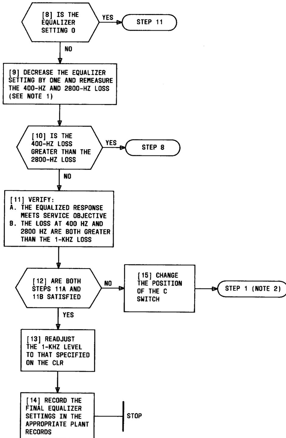
Fig. 10—Procedure for Equalizer Touch-Up (Sheet 2 of 2)
