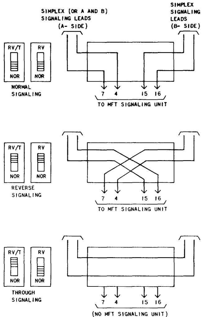
**Fig. 11 — Signaling Options for the J99343SC Repeater**
