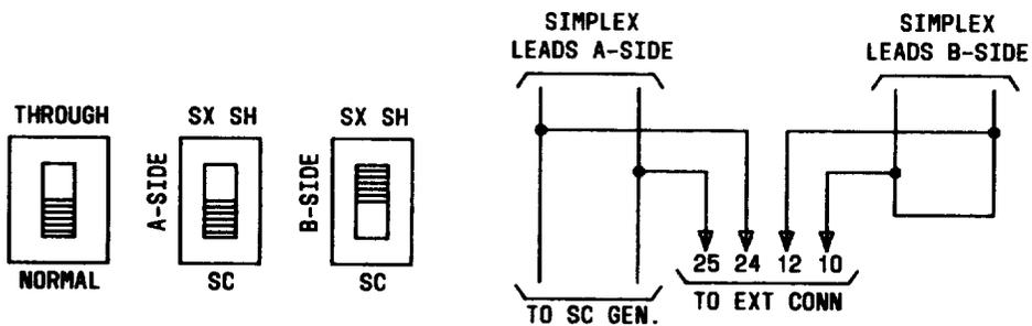
Fig. 15—Switch Settings for SD Repeater to Furnish A-Side Sealing Current
