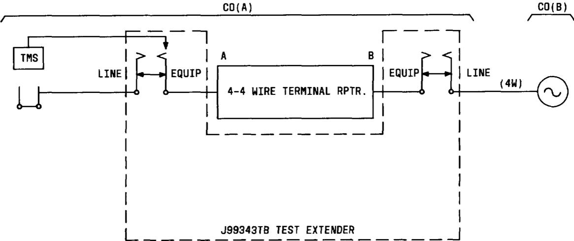
Fig. 7—Typical Test Configuration for Cable Loss—Terminal Repeaters
