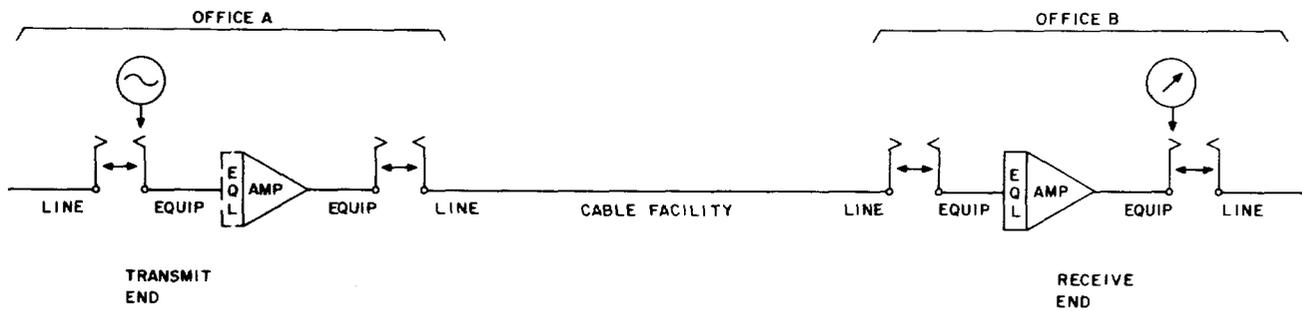
**Fig. 5—Typical Test Configuration for Cable Loss Frequency Measurements Using Multiple Repeater Section**
