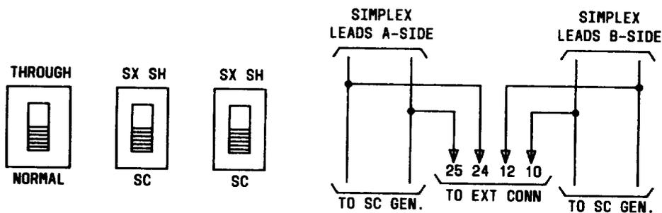
Fig. 16—Switch Settings for SD Repeater to Furnish A- and B-Side Sealing Current
