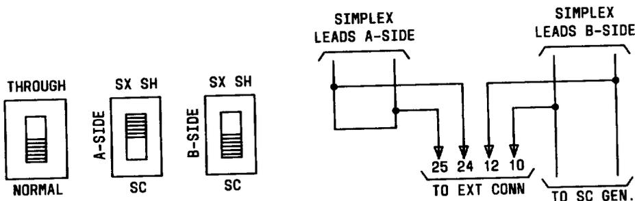
Fig. 14—Switch Settings for SD Repeater to Furnish B-Side Sealing Current
