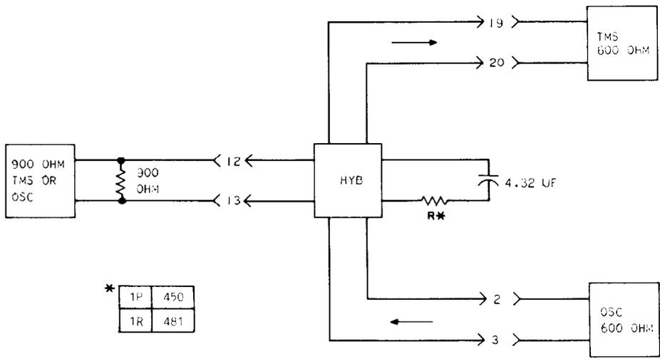
Fig. 3—1P/1R Terminating Set Transducer Characteristics
