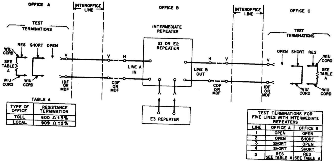
Fig. 5 — Test Terminations for Lines with Intermediate Repeaters — Manual Application Shown
