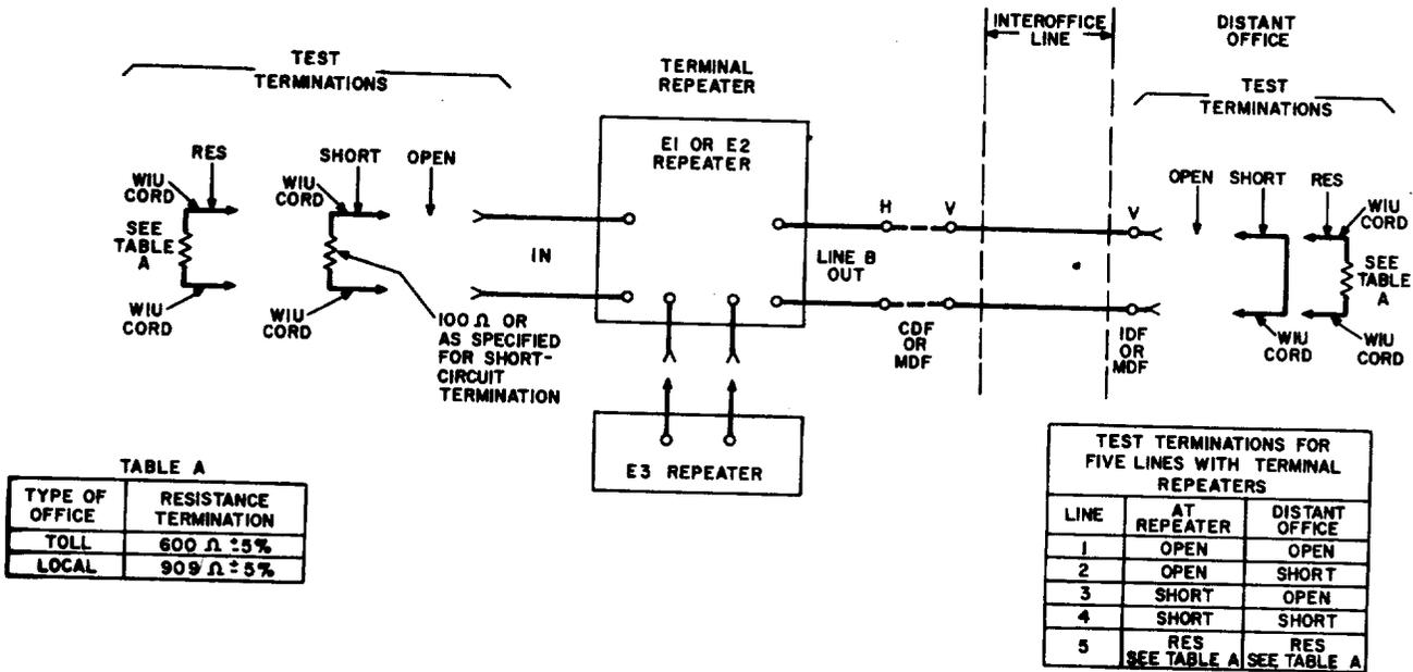
Fig. 6 — Test Terminations for Lines and Terminal Repeaters — Manual Application Shown
