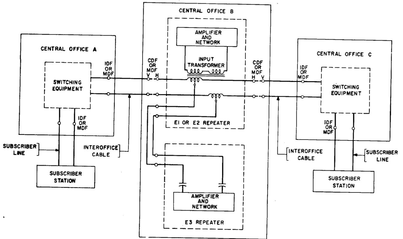
Fig. 1 — Typical Application of an Intermediate E13 or E23 Repeater
