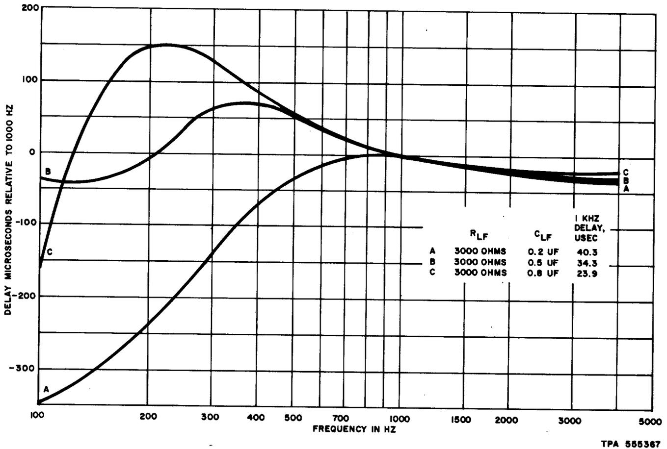
Fig. 14—359P Equalizer Low-Frequency Characteristics—Delay Between 600 Ohms, Varying CLF for RLF Constant at 3000 Ohms
