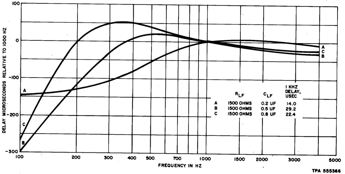
Fig. 13—359P Equalizer Low-Frequency Characteristics—Delay Between 600 Ohms, Varying  $C_{LF}$  for  $R_{LF}$  Constant at 1500 Ohms
