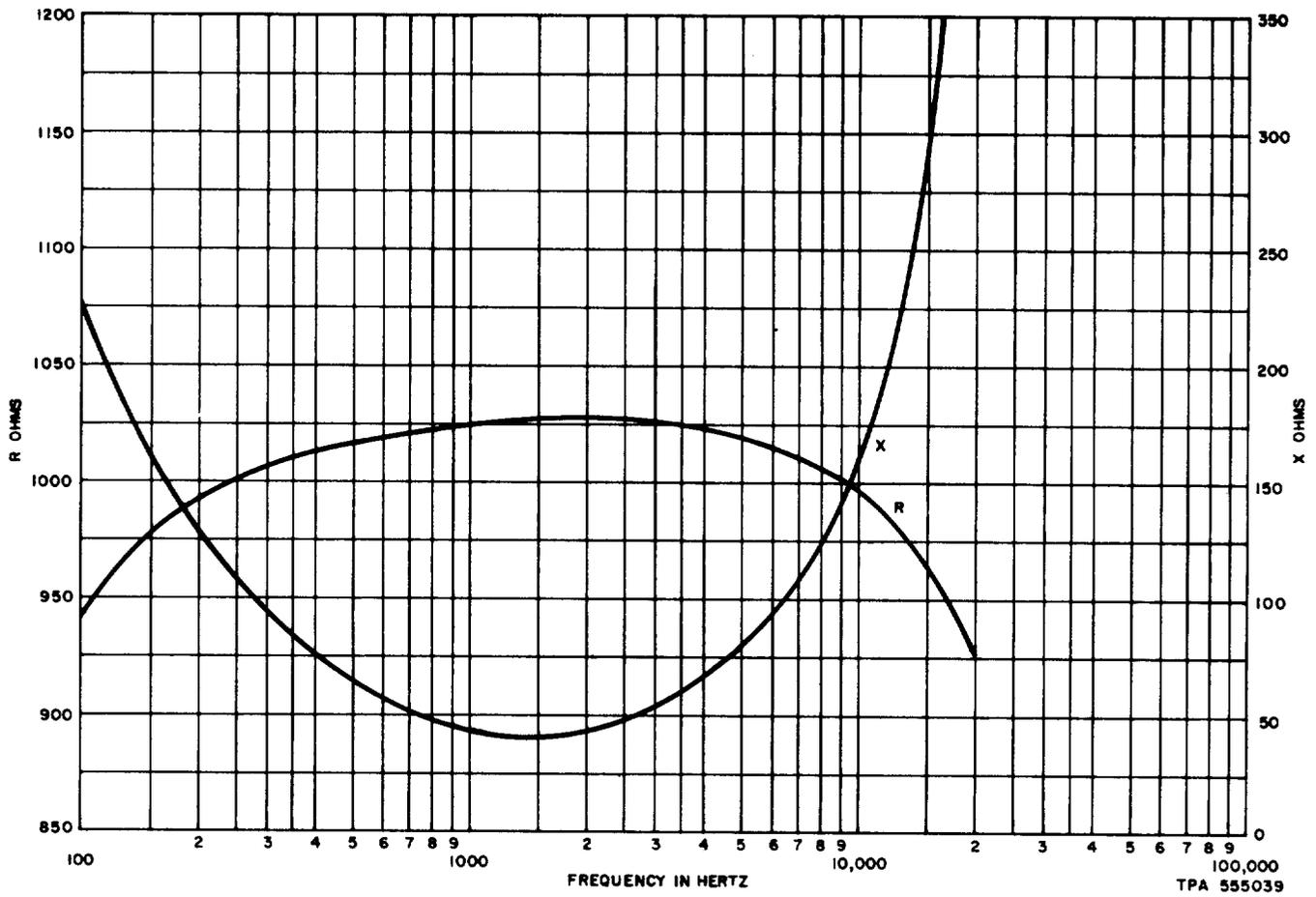
Fig. 7—F58122 Amplifier—Output Impedance—1200-Ohm Termination
