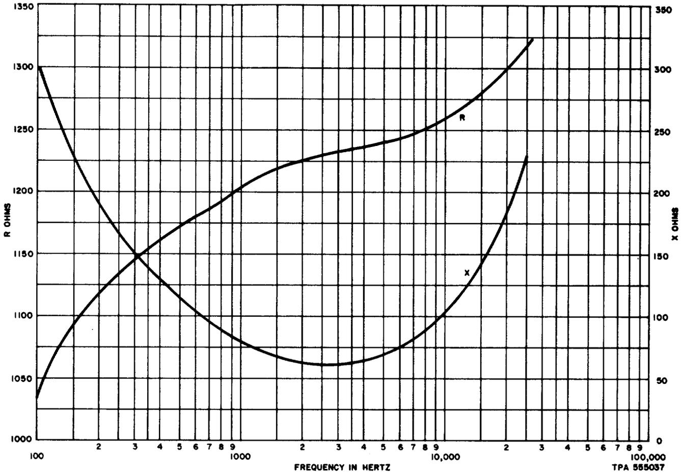
Fig. 5—F58122 Amplifier—Input Impedance—1200-Ohm Termination
