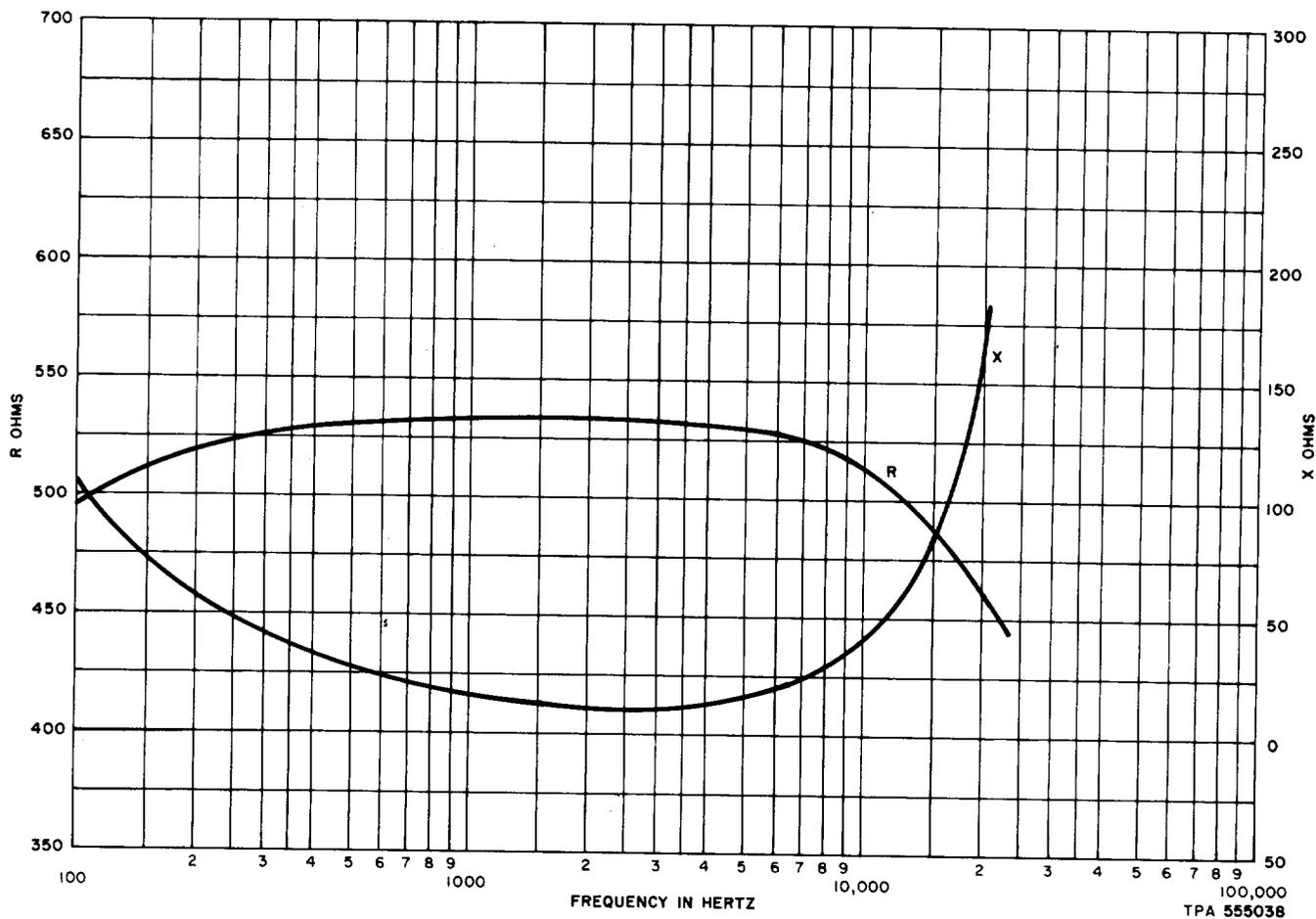
Fig. 6—F58122 Amplifier—Output Impedance—600-Ohm Termination
