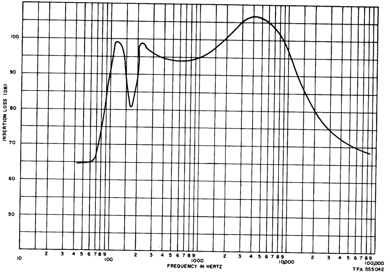
Fig. 10—F58122 Amplifier—Reverse Transmission Loss
