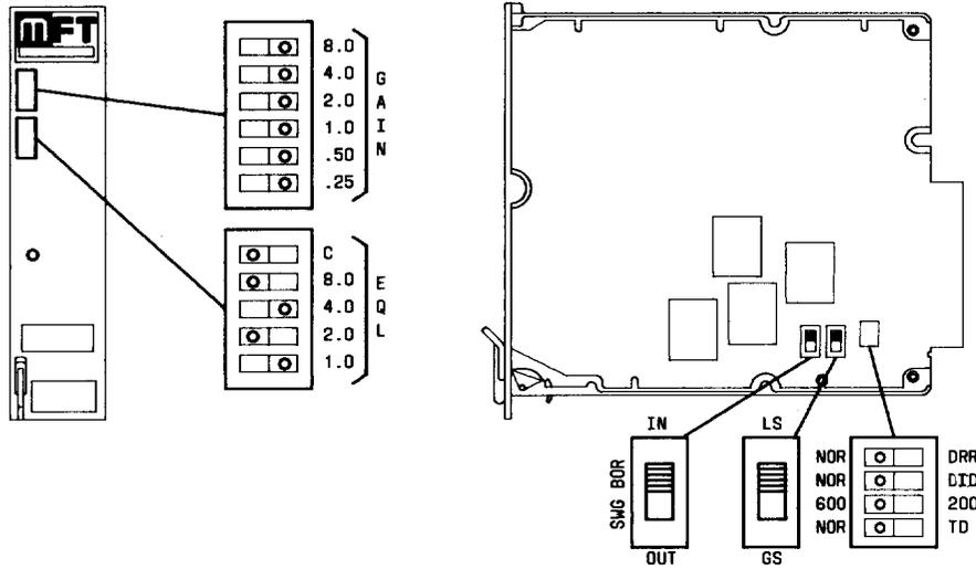
Fig. 2—J99343GS CFU—Switch Layout
