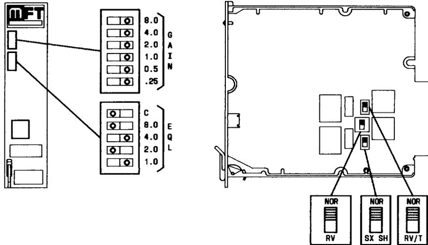
Fig. 2—J99343PR Repeater—Component Layout
