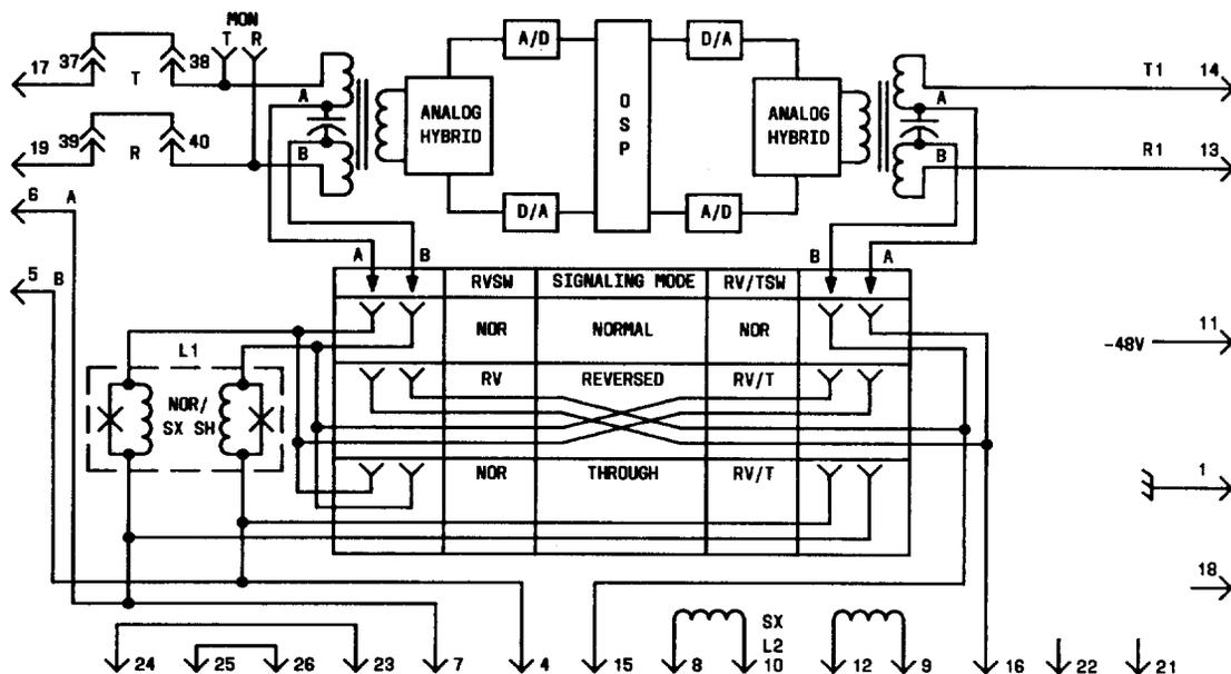
Fig. 1—Block Diagram of the J99343PR UA Repeater
