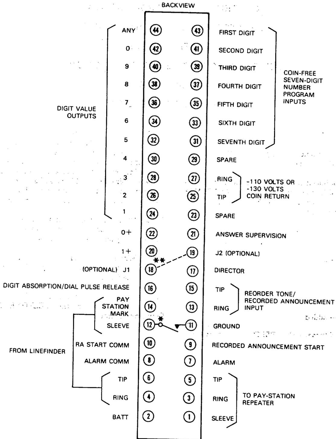
\* Pins 11 and 12 short together to automatically busy out the linefinder when the circuit card is not inserted into the connector.
