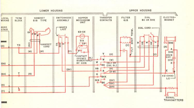
Fig. 1—Circuit Diagram of 210G, H; 212G, H; 193GN, HN; and 198GN, HN
