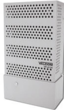
with respect to ground. The regulator will maintain 24 Volts +/- 2% over the rated range of input voltages and output loads. A greater than 4 Amp load on power up will cause the power supply to current limit. Short circuit protection is provided. Overvoltage is provided to limit the output voltage to approximately 28 Volts should a failure occur within the power supply. Outputs may be used in a series for 48V @ 2A.
