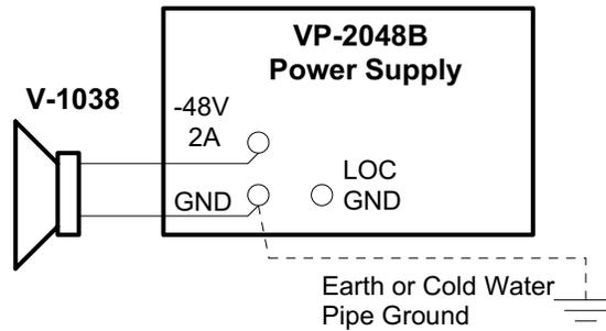
**Alternate Ground Method: If using earth or cold water pipe ground, do not connect to LOC GND.**
