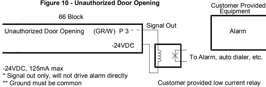
**Figure 11 - Remote Signalling Relay**
