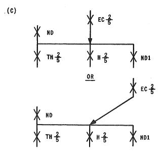
INDICATES H-RELAYS WILL NOT OPERATE UNTIL BOTH ND AND EC RELAYS HAVE OP-ERATED. ALSO THE ND1 AND THE RE-LAYS WILL OPERATE AFTER THE ND RELAY HAS OPERATED BUT INDEPENDENTLY OF THE EC & RELAYS.
