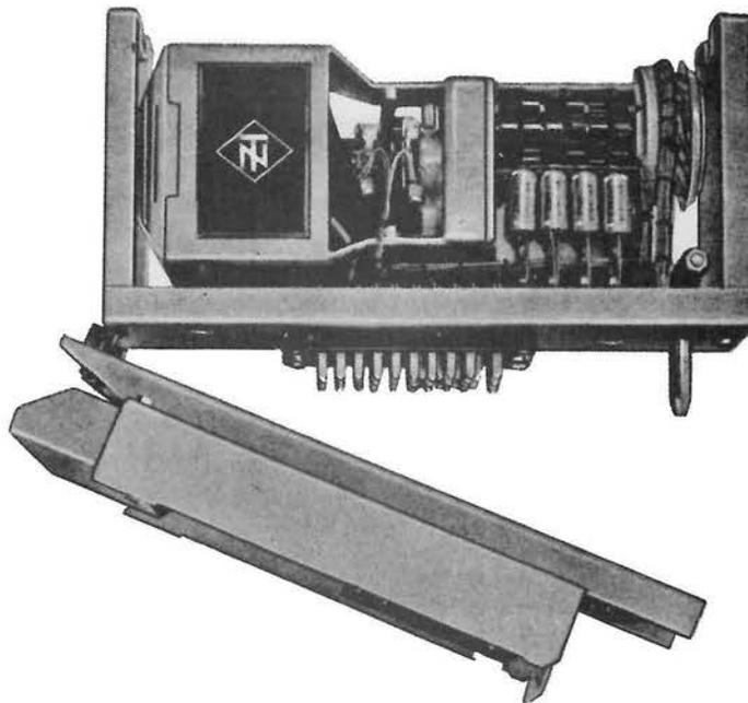
Fig. 7 ringing current and tone generator with adapter.
