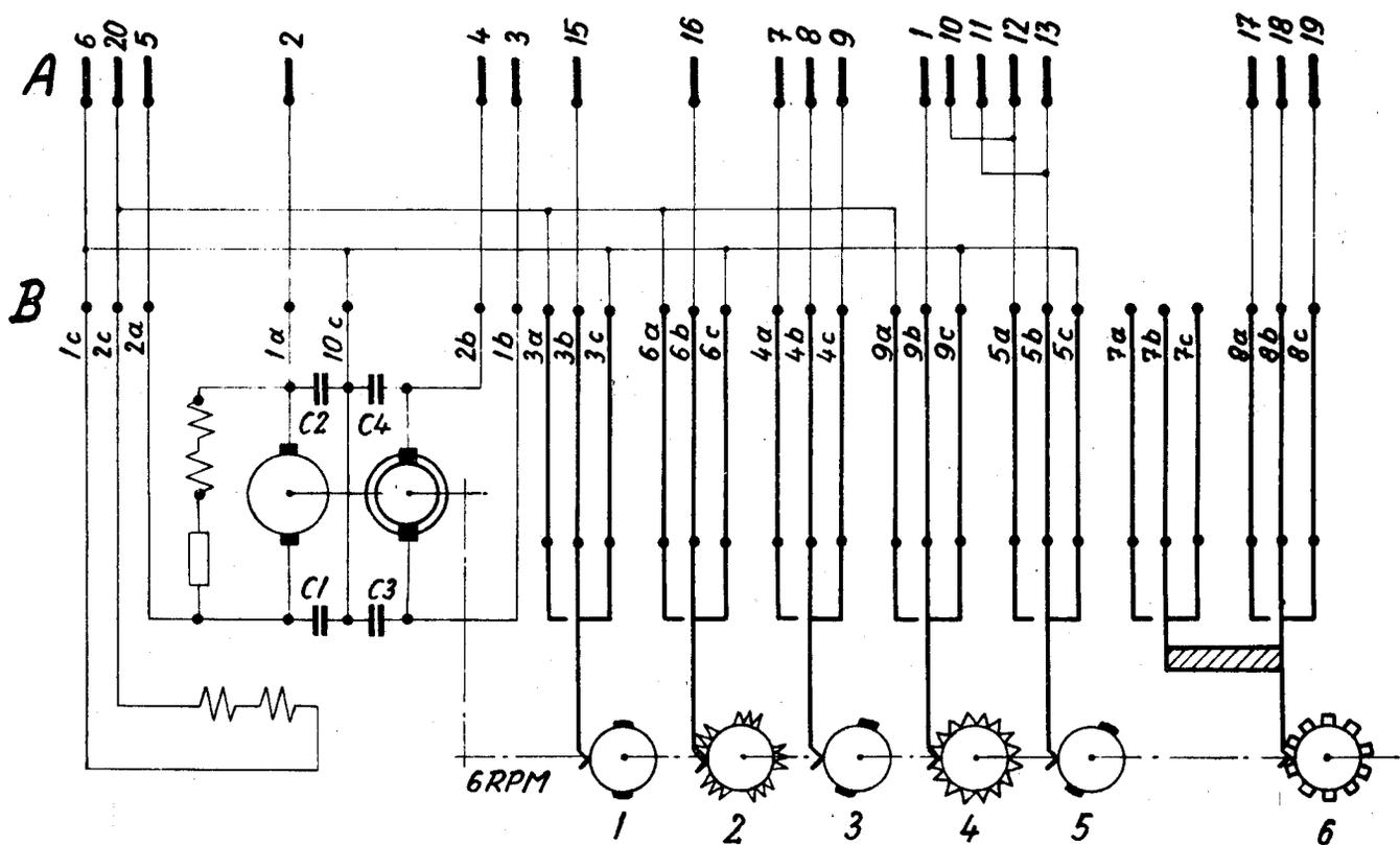
Fig. 8 Diagram of ringing current and signal generator
