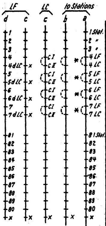
\* Remove straps for connection of auxiliary equipment (a, b, c, d from LC for search-seize or answering numbers.
