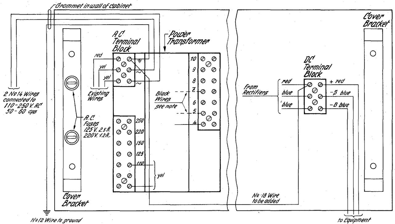
**Important:** Fuses - For Connection to 110-150 V. AC: 2.5 A.
