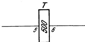
T identifies the relay. The DC resistance of the winding is 500 ohms and the winding is connected to terminals 5 and 6.
