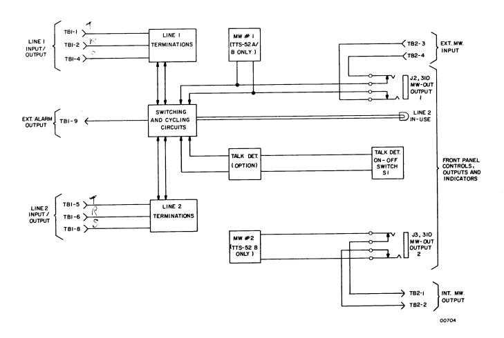
Figure 4-3. TTS 52 Overall Block Diagram
