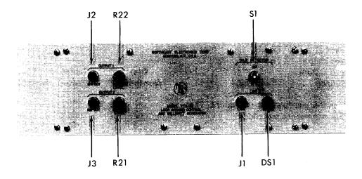
Figure 3—1. TTS 52 Controls, Indicators and connectors.
