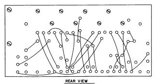
Figure 8-3. TTS 50XS Main Circuit Board, Component Location Diagram
