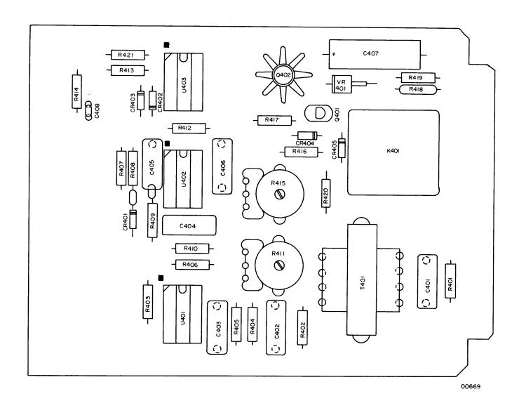
Figure 6-3. TTS 52 Talk Detector Circuit Board, Component Location Diagram
