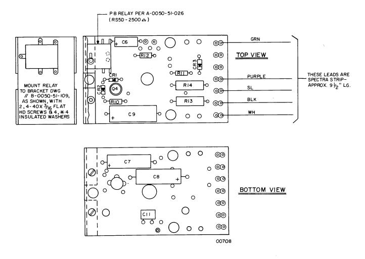
Figure 8-5. TTS 50XS FP Selective Detector, Component Location Diagram (2 of 2)
