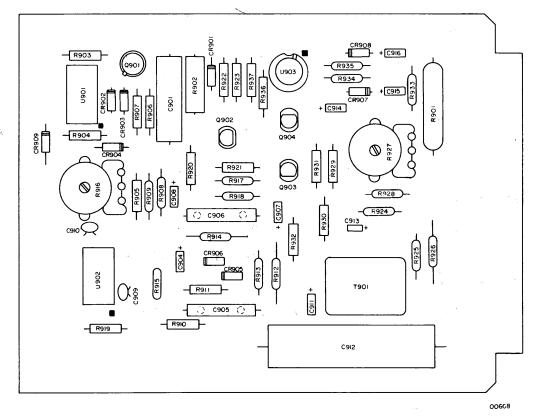
rigure 6-2. TTS 52 Milliwett Generator Circuit Board, Component Location Diagram
