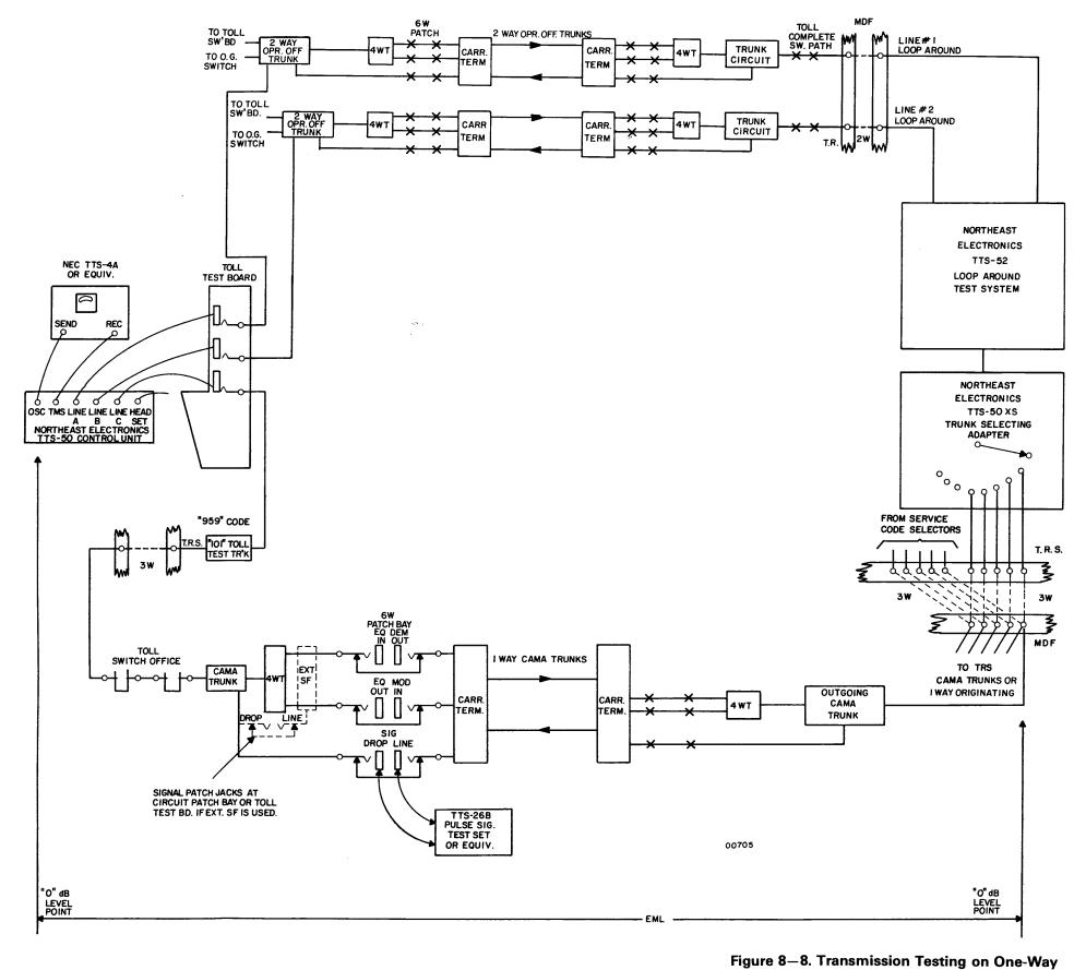
CAMA Trunks Using TTS 52 and TTS 50XS
