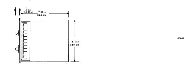
Figure 3-2. TTS 52 Overall Dimensions
