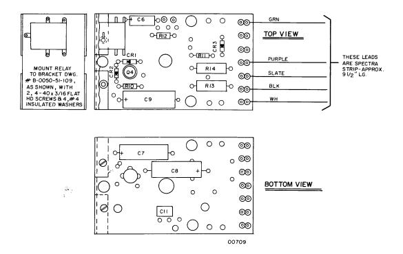
Figure 8-4. TTS 50XS FQ Selective Detector, Component Location Diagram (2 of 2)
