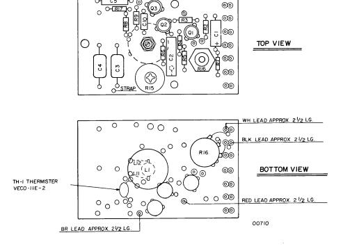
Figure 8-4. TTS 50XS FQ Selective Detector, Component Location Diagram (1 of 2)
