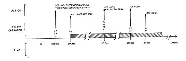
Figure 4-2. TTS 52 Line 2 Timing Diagram
