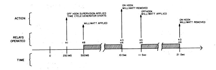
Figure 4-1, TTS 52 Line 1 Timing Diagram
