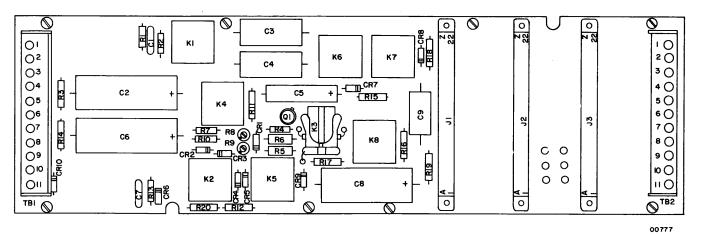
Figure 6-1. TTS 52 Main Assembly Circuit Board, Component Location Diagram
