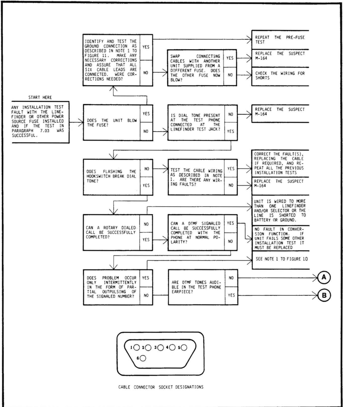
Figure 13 Installation Test Post-Fuse Faults (Sheet 1 of 4)
