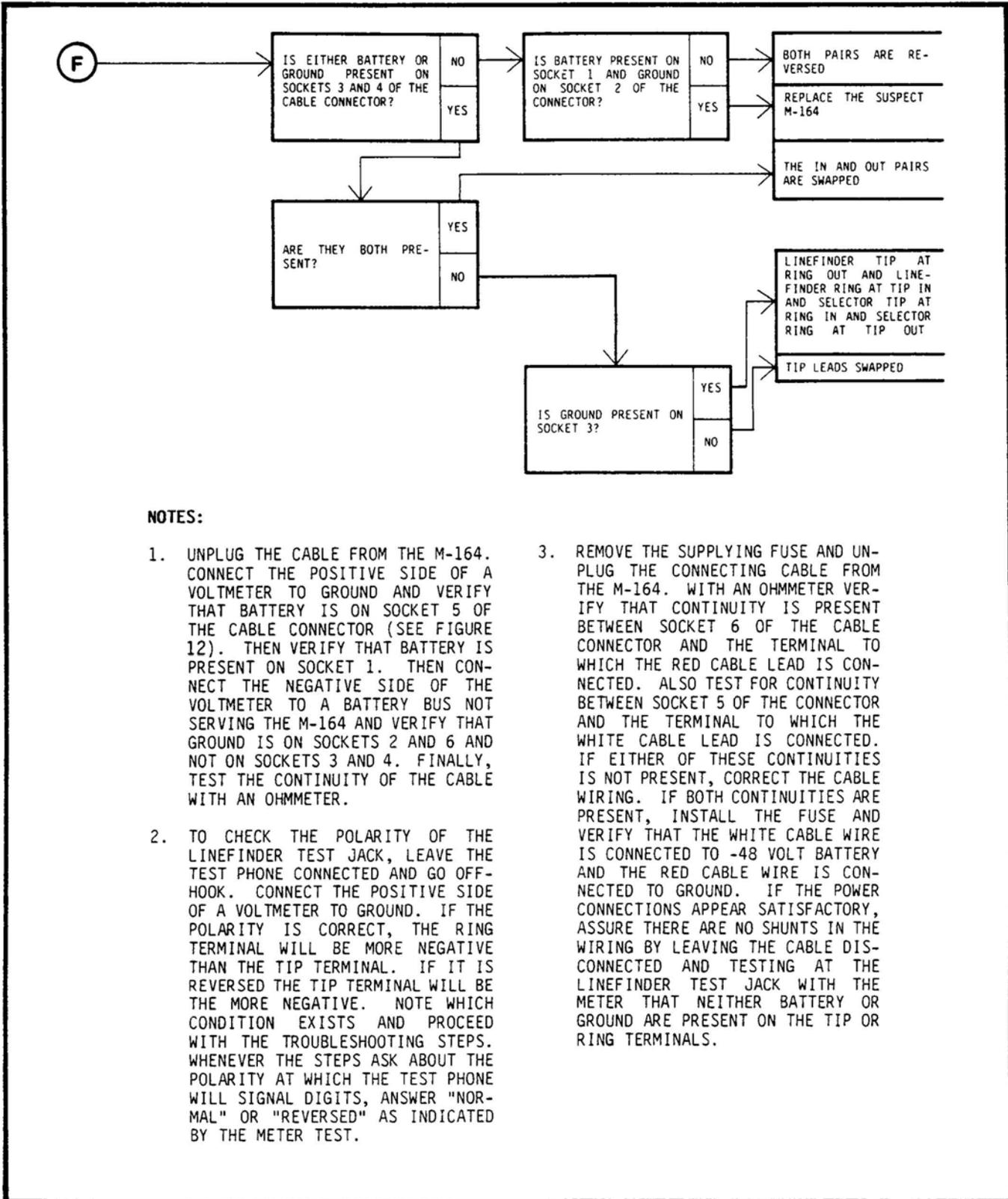
**Figure 13 Installation Test Post-Fuse Faults (Sheet 4 of 4)**
