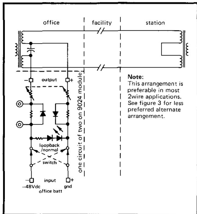
figure 2. Single circuit of 9024 in 2wire application (preferred arrangement)
