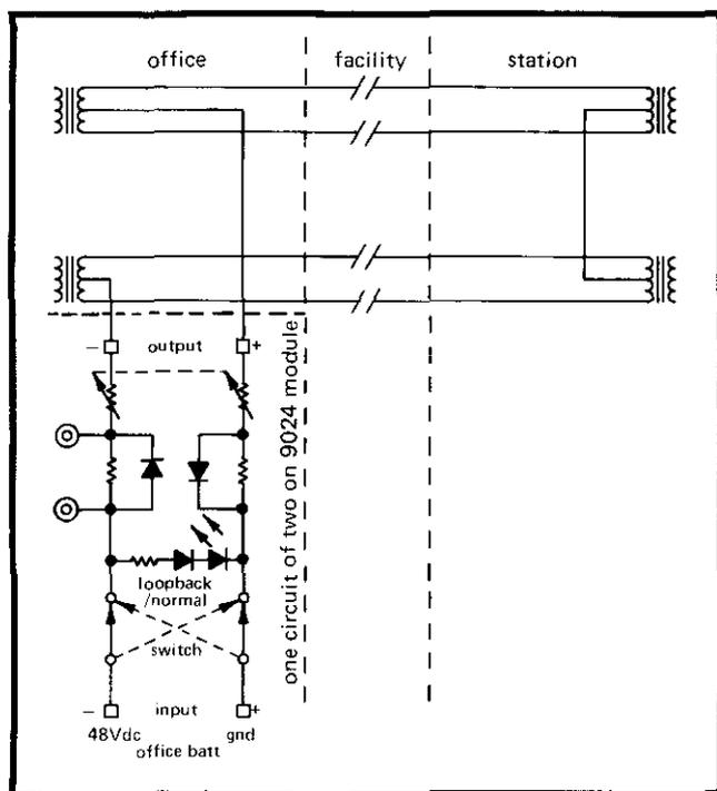
figure 4. Single circuit of 9024 in 4wire application
