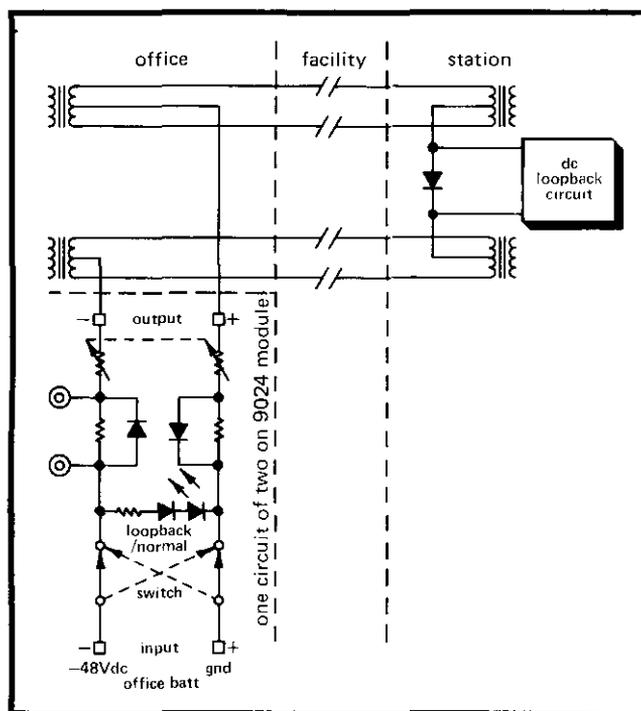
figure 5. Single circuit of 9024 in 4wire application with loopback
