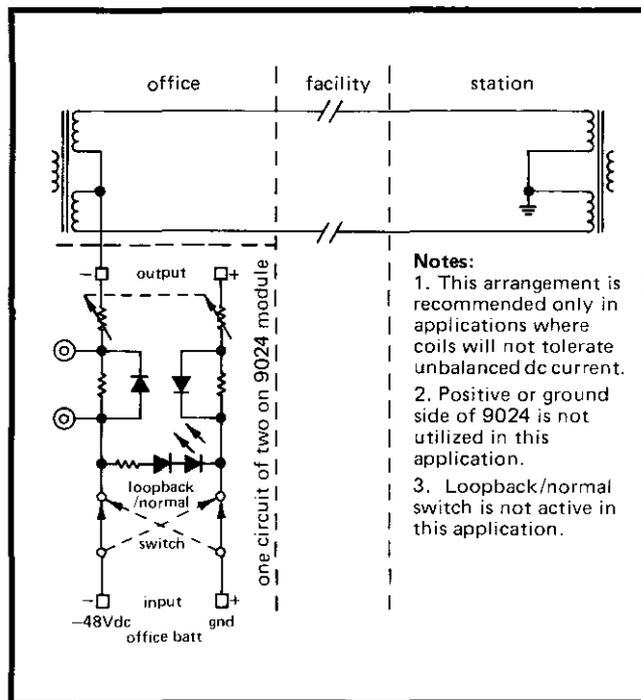
figure 3. Single circuit of 9024 in 2wire application (alternate arrangement)
