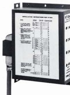
**KT-364 Four Area Pager:** Provides paging capability for one to four areas by dial accessing the four 5-watt amplifiers individually or in combinations. Features access circuitry, volume control, visual busy indication, background music input and 8-ohm output impedance.
