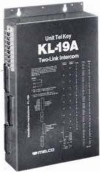
**KL-19A Two-Link Intercom System:** Equips up to 19 stations with two talking paths, call progress tones, flashing lamps, interrupted ringing and conferencing. One of the talking paths is private, the other is common. Both links and all stations are accessed from one telephone pickup key at each station. The system can easily be adapted for paging, and system capacity can be expanded to 38 stations by adding a Melco KX-38 Intercom Expander.
