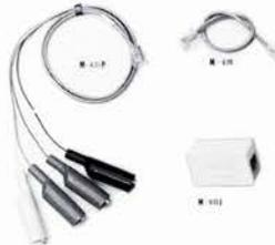
**M-621P, M623J & M-629:** The M-621P and M-629 Modular Wiring Test Cords and the M-623J Modular Connector are designed to provide convenient connections between the M628-1 Power Supply and the modular wall jack. The M-629 is a male modular to male modular cord, the M-621P is a male modular plug to alligator clip cord, and the M-623J is a female modular connector/adaptor.
