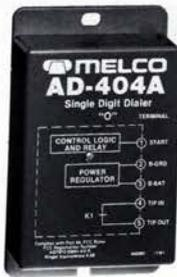
**AD-404A Single Digit Dialer:** Dials "0" to summon the operator for assistance when it detects an off-hook signal. Functions on any line capable of registering dial pulses. The AD-404A requires A-A1 wiring and a 24-volt power supply.
