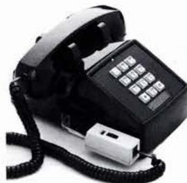
**NEW S-11M Modular Telephone Amplifier (Magniphone):** A user-installable amplifier which can be used with any single-line modular telephone. Connects to the telephone in just a few seconds by plugging the handset cord into the S-11M jack and inserting the S-11M plug into the modular telephone jack. Individually packaged for retail display, the S-11M operates in the same manner as the S-11.
