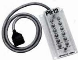
**PB-12 Power Block Assembly:** Designed for use at key system installations where a modular power supply is in place and power distribution by individual conductors is required. The PB-12 consists of a connector, a 12-conductor cable and a terminal block with 12 screw terminals. It mounts easily on a backboard, on a relay rack or in an apparatus cabinet.
