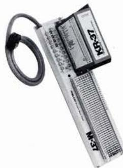
**M-37 Modular Panel:** Provides rapid mounting for Melco 10, 19 and 37-station intercoms. Minimum wiring changes are necessary when a 10 or 19-station intercom is replaced with a larger one. An optional plug-ended power cable, the CA-12, is available for connections with a modular power supply.
