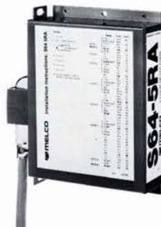
**S64-5RA Loop Detector:** Provides five loop sensing circuits which can be used in the same applications as the S64-1. The S64-5RA is contained in an aluminum housing with a plug for convenient connections to a 25-pair connector cable.
