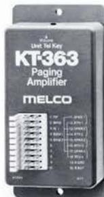
**KT-363 Paging Amplifier:** Provides access to a paging area through a 10-watt amplifier. The KT-363 has access circuitry, volume control, background music input and 8-ohm output impedance to speakers.
