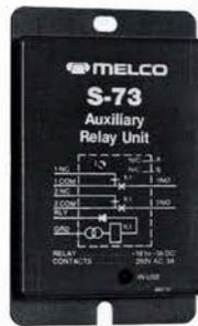
**S-73 Auxiliary Relay Circuit:** A general purpose relay circuit which can be used for various transfer functions. The relay operates from either a ground or battery input of 18 to 56V DC, and an LED lights when the relay is operated.
