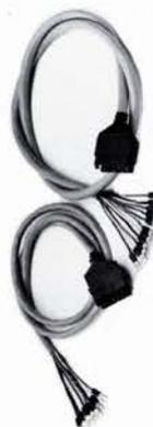
**CA-7 & CA-12 Power Cable Assemblies:** Provide power connections from a W.E. Co. 79B1, 90B2 or similar modular power supply using connectors and plugs. Both have a plug on one end and spade-ended conductors on the other. The CA-7, with 7 conductors, is designed for use with Melco's M-19 Modular Panel, MP-610 Key System Panel and KL-30 Two-Link Intercom System. The CA-12, with 12 conductors, can be used with Melco's M-37 Modular Panel.
