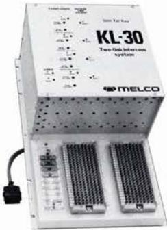
**KL-30 Two-Link Intercom System:** Provides up to 40 stations with two private talking paths, call progress tones, flashing lamps, interrupted ringing and lockout. Only one telephone pickup key is required to access all stations and both links. Switch-selectable PABX features include specific call pickup, call forwarding, conferencing, message waiting and do-not-disturb. Paging, outside line access and call announcing capabilities are circuit pack options.
