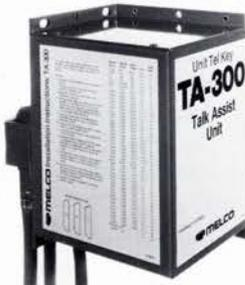
**TA-300 Talk Assist Unit:** Operates in conjunction with the KM-330B, allowing for a service observer to enter the conversation on the line being observed and offer immediate assistance. The talk assist feature is easily accessed by depressing an assigned pushbutton on the service observing telephone. Each TA-300 added to the KM-330B system provides talk assist capability for 30 lines.
