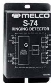
**NEW S-74 Ringing Detector:** A multi-application ringing detector that operates a relay circuit when ringing voltage is present. It can be used to activate an auxiliary visual or audible device, or to provide bridged ringing for an off-premise extension. The S-74 mounts on a backboard, connects from screw terminals and operates from either a 15 to 18V AC wall pack or a standard key system power supply.
