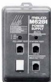
**M628-1 Modular Wiring Power Supply:** A battery operated power supply which simulates central office battery and local lamp transformer power in modular station installations. It can be used to test C.O. line conditions, or to test station wiring in conjunction with the M-630.
