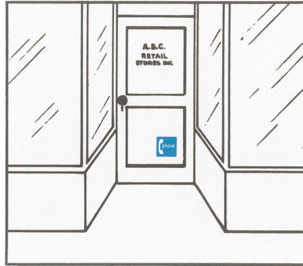
Poor placement: sign is visible from too small a viewing angle
