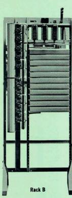
KMG 50: A maximum capacity of 50 extension lines with 6 conversation links; The KMG 50/6 consists of Rack "A" shown above and may be expanded later to 100 extension lines by the addition of Rack "B" shown above.
