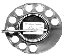
FIGURE 2: TO REMOVE NUMBER CARD RING:
