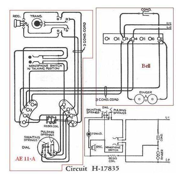
Externally, the AE 11-A is identical to the AE 1-A but the 11-A uses a different receiver element and is a complete telephone except for a bell. The anti-side tone circuit of the 11-A uses the special receiver element. The receiver is un-biased (there is no magnet) and required a DC current to bias it.
