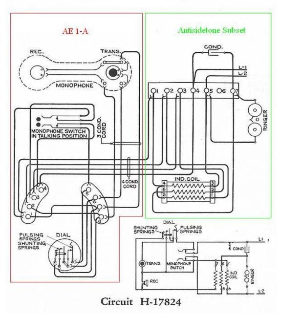
Shown above is the AE 1-A and its circuit. The AE 1-A is designed to work with an anti-side tone subset such as the Type 21.
