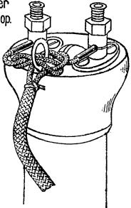
Pull conductors tight and connect tips to binding posts.
