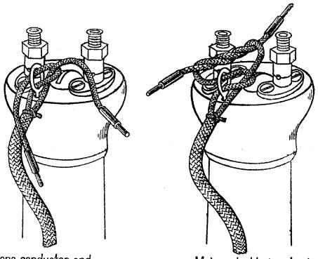
Loop one conductor and pass the loop through the screw eye. Pass the other conductor through the loop.
