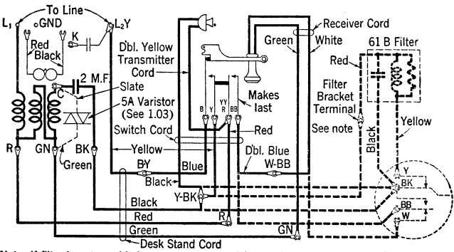
Note: If filter is not provided connect yellow lead from switchhook to Y of dial instead of to filter bracket terminal.
