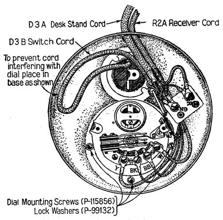
After passing open ends of cord stay hooks through hole in bracket, pinch openings together with pliers.
