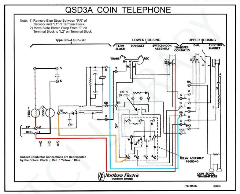
Fig. 3 - Circuit Diagram for Connecting QSD3A Coin Collector to NE-685A Network Type Subset
