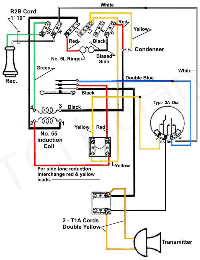
N.B. - If a louder ringer is required, disconnect the 6-L ringer and connect a type 392-J Subscriber set to terminals "L-1" and "C".
