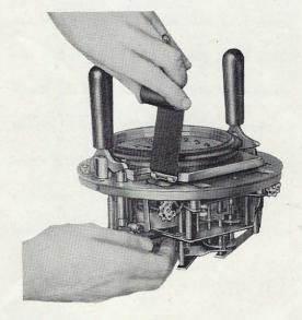
Press the open side of hook gently up against ribbon spool with finger of one hand, then with thumb and finger of the other hand, slowly turn the spool in the direction shown by arrow, until the flange on the inner heel of hook falls into groove in spool; when this occurs, a little extra pressure against the hook will cause it to snap over the spool, where it will be firmly held in its proper position.
