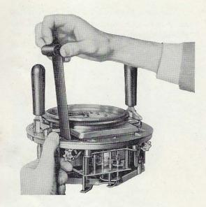
Now turn the thumb wheel in direction as shown by arrow, winding up all the ribbon except about 9 inches.
