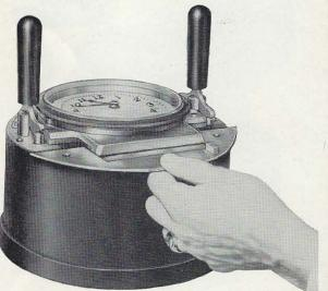
Lift instrument out of case by the two handles.
