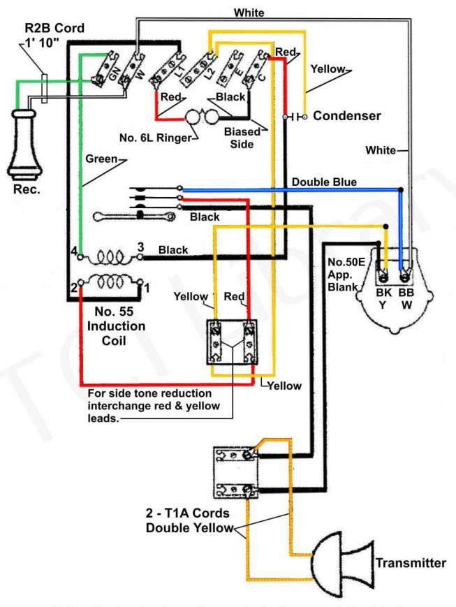
N.B. - If a louder ringer is required, disconnect the 6-L ringer and connect a type 392-J Subscriber set to terminals "L-1" and "C".
