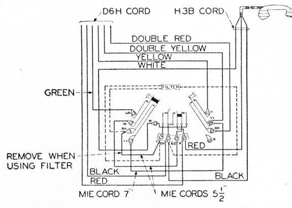
The No. 203 Type Hand Telephone Set is designed for use at anti-sidetone two-party selective message rate, party on tip stations in dial systems.
