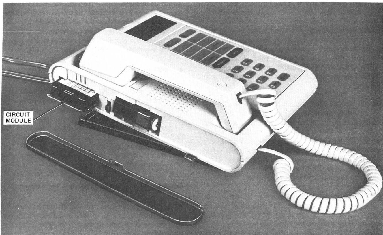
Fig. 2—Circuit Module Installation (Console)
