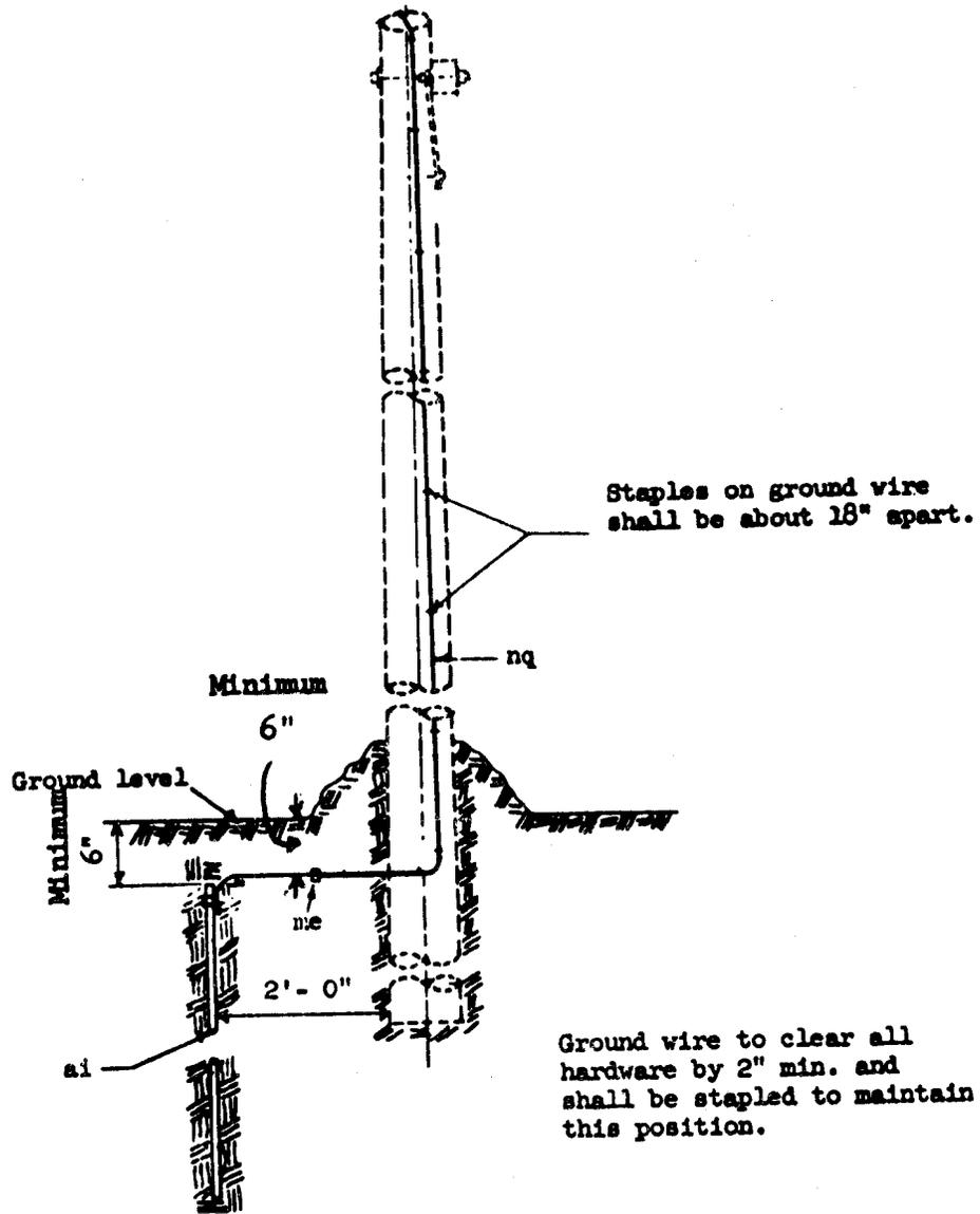
USED PRIMARILY ON NON-JOINT POLES TO PROVIDE A GROUND FOR POLE OR CROSSARM-MOUNTED LIGHTNING ARRESTERS AND FOR DRAINAGE UNITS. FOR APPLICATIONS SEE REA TE & CM-830, "SUMMARY OF UNITS FOR ELECTRICAL PROTECTION."
