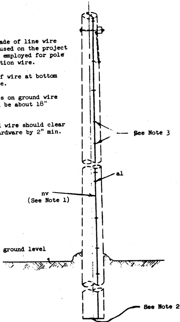
USED TO PREVENT SPLITTING OF WOOD POLES BY LIGHTNING IN AREAS OF HIGH LIGHTNING INCIDENCE. SEE REA TE & CM-820, "OPEN WIRE CIRCUIT PROTECTION," FOR APPLICATION.
