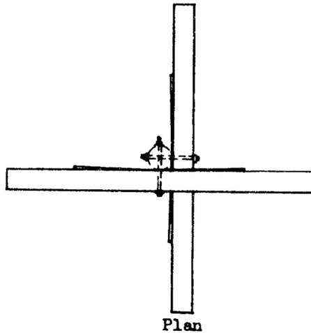
USED ON JOINT OR NON-JOINT CORNER POLES. LIMITATIONS: CORNERS 60 TO 90 DEGREES. MAXIMUM LONGITUDINAL PULL 650 LBS. PER CONDUCTOR. WHERE DEADENDING ONLY 4 TO 6 WIRES WITH THE REMAINING PIN POSITIONS NOT TO BE OCCUPIED ULTIMATELY, THE MAXIMUM LOAD PER WIRE MAY BE PROPORTIONALLY INCREASED. NOT TO BE USED ON LINES USING REA-1 TRANSPOSITION SYSTEM. SEE FIGURES 36, 37, AND 38 FOR THESE EXCEPTIONS. SEE GUIDE DRAWING 702 FOR NOTE ON CLIMBING SPACE.
