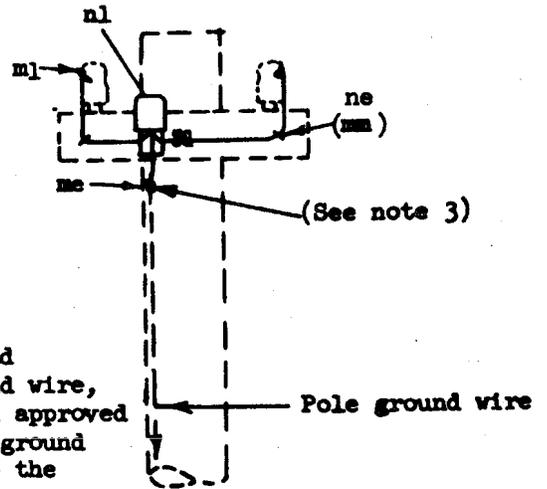
USED ON AN OPEN WIRE TELEPHONE CIRCUIT FOR PROTECTION AGAINST POWER CONTACTS. SEE REA TE & CM-820, "OPEN WIRE CIRCUIT PROTECTION," FOR APPLICATIONS.
