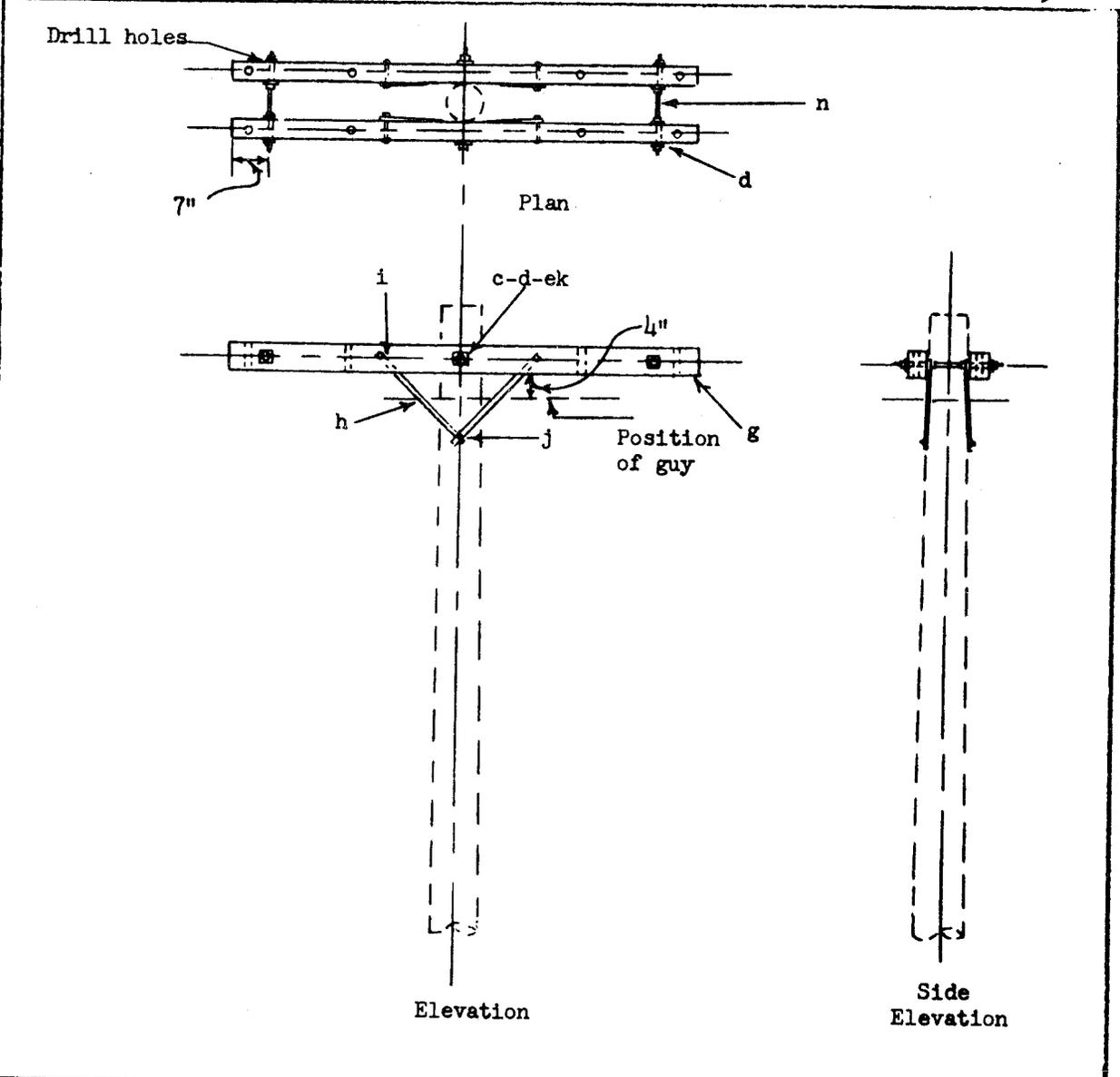
USED ON NON-JOINT TANGENT OR CORNER POLES. LIMITATIONS: MAXIMUM CORNER 35 DEGREES; 225 LBS. MAXIMUM VERTICAL LOAD PER CONDUCTOR; 10 PERCENT MAXIMUM DOWNWARD GRADE CHANGE.
