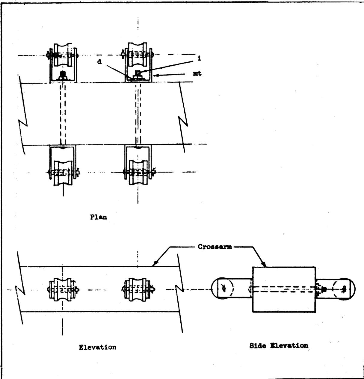
USED FOR DEADENDING CIRCUITS IN BOTH DIRECTIONS ON A CROSSARM AND THE WIRE PULL ON EACH INSULATOR KNOB WILL NOT EXCEED 1500 LBS; ALSO FOR DEADENDING BOTH WAYS WHERE DOWNWARD PULL EXCEEDS 25 PERCENT. SEE PBl-6 and PBl-7 AND GUIDE DRAWINGS 165 AND 165-1.
