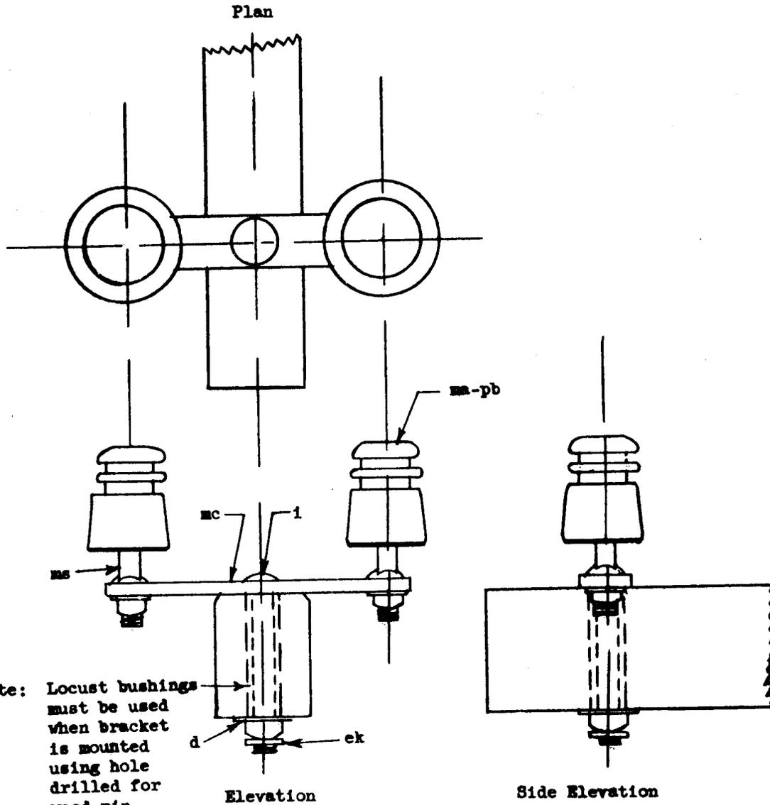
Note: Locust bushings must be used when bracket is mounted using hole drilled for wood pin.
