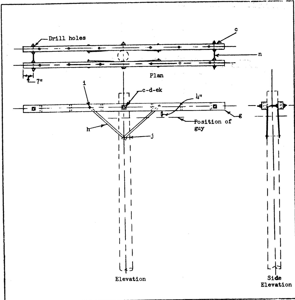
USED ON NON-JOINT OR JOINT TANGENT OR CORNER POLES FOR 4 INCH SPACED INSULATED OPEN WIRE USING T-21 STEEL BRACKET UNITS FOR WIRE ATTACHMENTS; AT ALL RAILROAD AND RIVER CROSSINGS; AND AT DOWNWARD GRADE CHANGES EXCEEDING 10 PERCENT. LIMITATIONS: CORNERS 35 TO 60 DEGREES: MAXIMUM VERTICAL LOAD PER CONDUCTOR 450 LBS.; AND 25 PERCENT MAXIMUM DOWNWARD GRADE CHANGE. SEE FIGURE 11 FOR WIRE ATTACHMENT METHODS.
