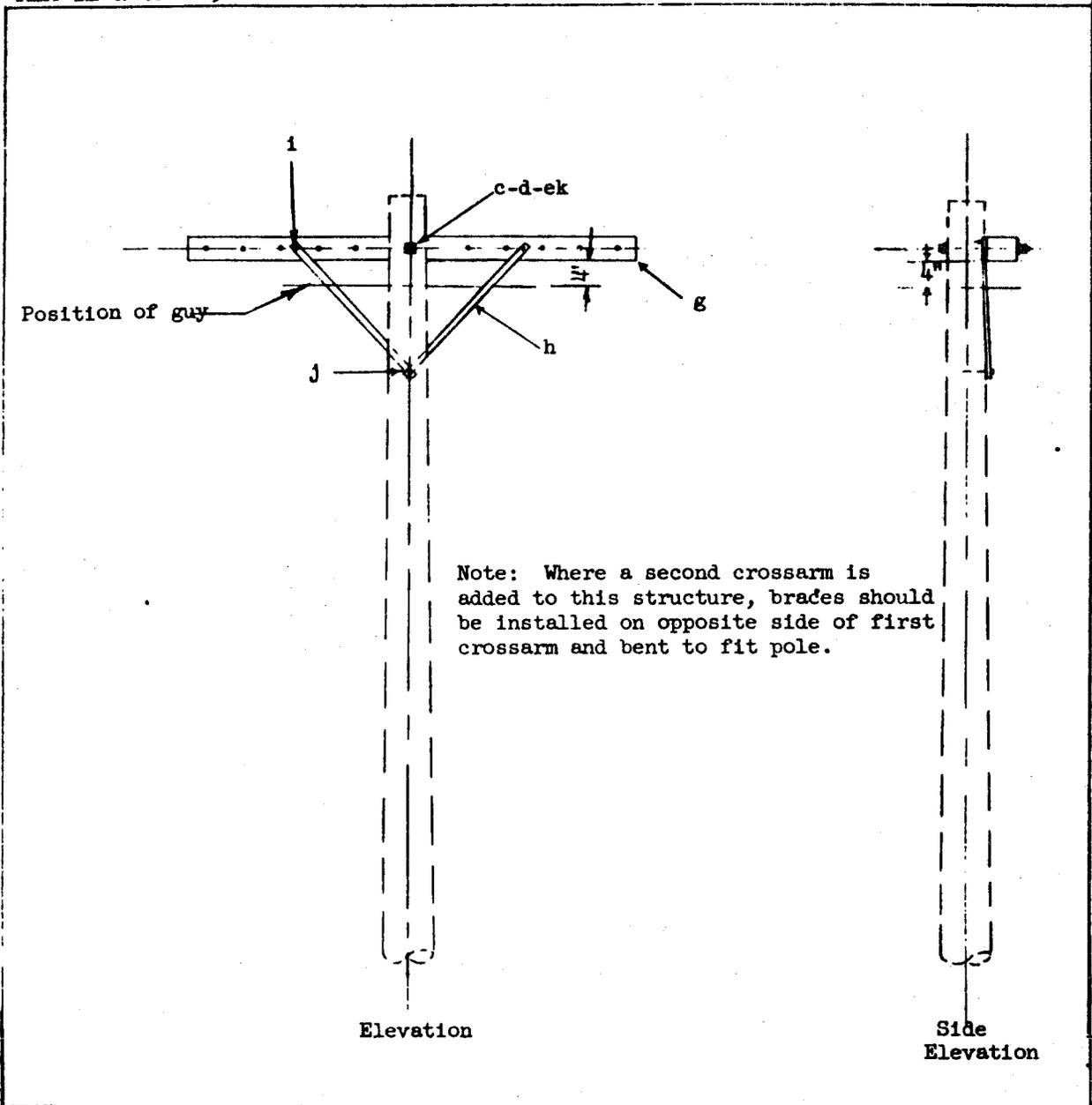
USED ON JOINT OR NON-JOINT DEADEND POLES. LIMITATIONS: MAXIMUM LONGITUDINAL PULL PER CONDUCTOR 650 LBS. WHERE DEADENDING ONLY 4 OR 6 WIRES WITH THE REMAINING PIN POSITIONS NOT TO BE OCCUPIED ULTIMATELY, THE MAXIMUM LOAD MAY BE PROPORTIONATELY INCREASED; AND NOT TO BE USED IN LINES USING THE REA-1 TRANSPOSITION SYSTEM. SEE FIGURES 36, 37, AND 38 FOR THESE EXCEPTIONS.
