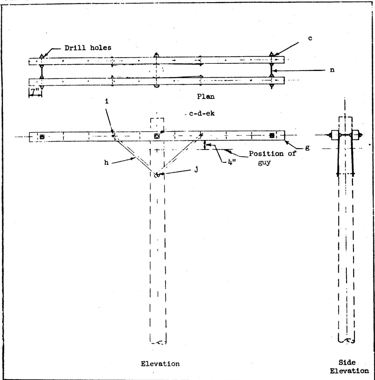
USED ON NON-JOINT POLES AT ALL RAILROAD AND RIVER CROSSINGS; ALSO AT CORNERS AND FOR DOWNWARD GRADE CHANGES EXCEEDING 10 PERCENT. LIMITATIONS: CORNERS 35 TO 60 DEGREES; VERTICAL LOAD PER CONDUCTOR 225 TO 450 LBS., AND 25 PERCENT MAXIMUM DOWNWARD GRADE CHANGE.
