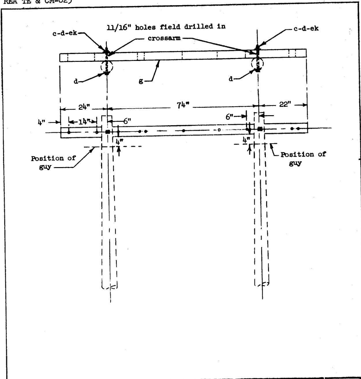
USED FOR DEADEND IN NON-JOINT LINE TRANSPOSED ACCORDING TO REA TE & CM-463, "REA-1 TRANSPOSITION SYSTEM," AS INDICATED ON FIGURE 3 THEREIN. IN TWO-CROSSARM CONSTRUCTION THE LOWER CROSSARM SHALL BE PLACED SO THAT THE 14 INCH PIN SPACING IS OPPOSITE (END-FOR-END) FROM THAT OF THE TOP CROSSARM.
