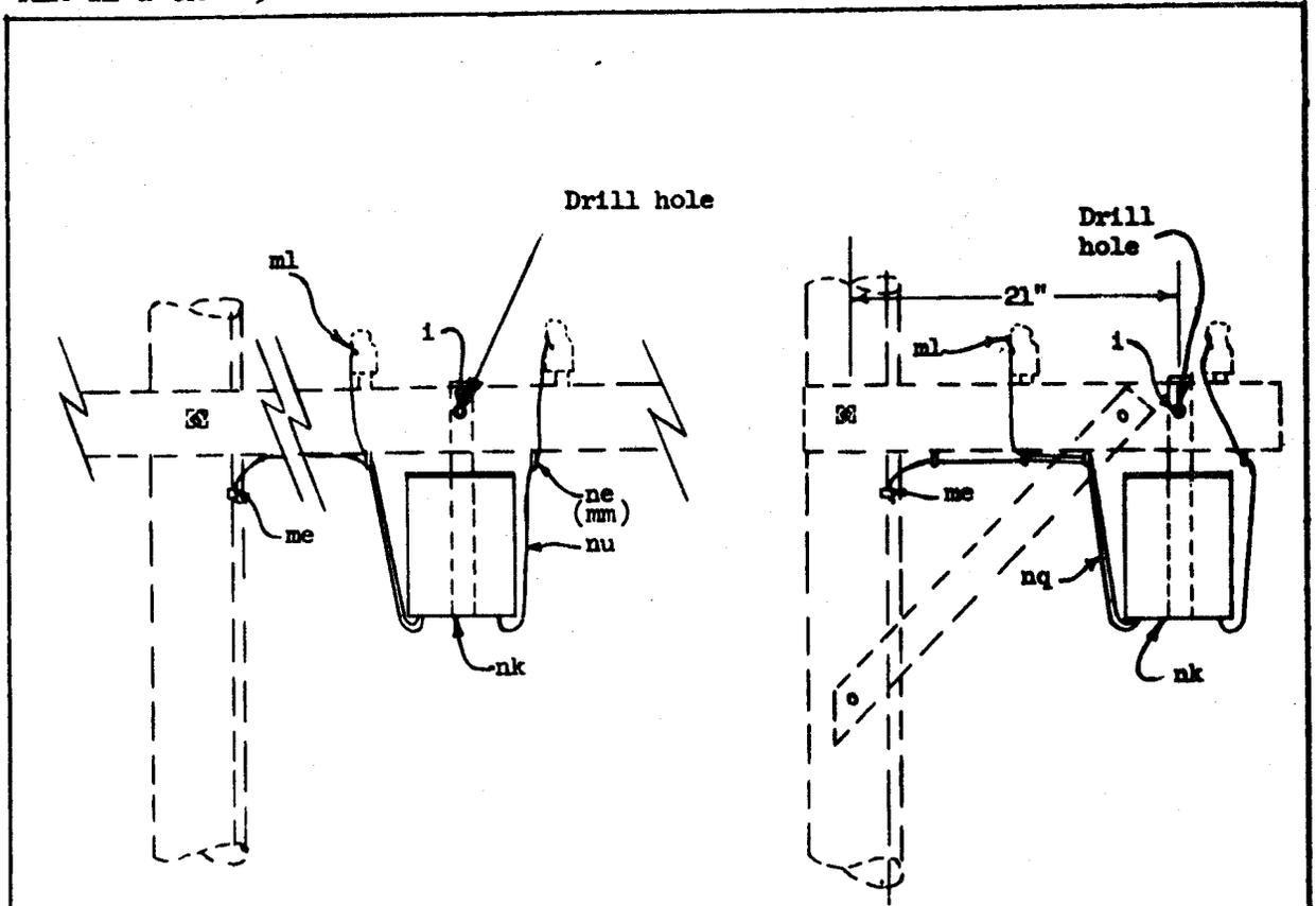
Note: If pole is not already equipped with a vertical pole ground wire, leave enough length of #10 AWG copper ground wire (item "nq") coiled and taped so that it may be extended up the pole and connected to a multigrounded neutral by a representative of the power company.
