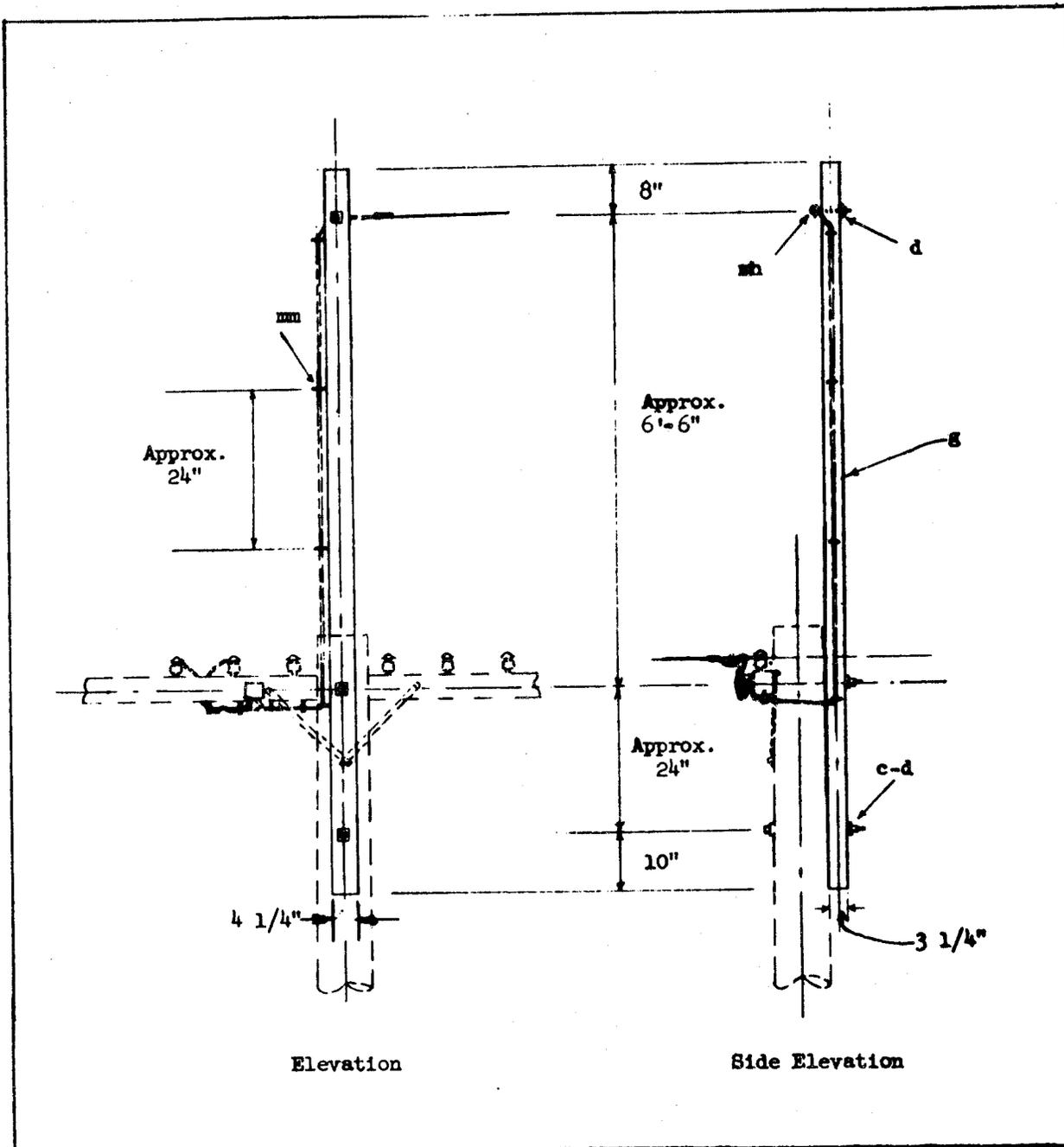
USED ONLY ON EXISTING POLES WHERE NECESSARY TO OBTAIN GROUND CLEARANCE FOR DROP WIRES ACROSS A HIGHWAY. THE CROSSARM MUST BE BORED ON THE JOB FOR THE POLE MOUNTING HOLES. TYPE 10A OR 10B CROSSARMS CAN BE USED FOR THIS UNIT. IN A NEW LINE THE POLE SELECTED SHOULD HAVE PROPER HEIGHT TO PROVIDE REQUIRED DROP WIRE GROUND CLEARANCE TO AVOID USE OF THIS UNIT.
