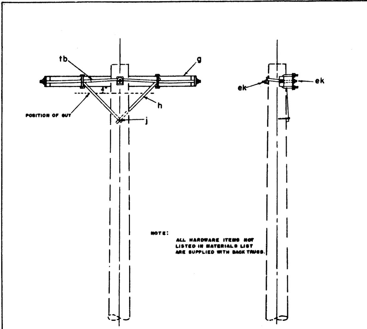
USED AS DEADENDS IN JOINT OR NON-JOINT CONSTRUCTION TRANSPOSED ACCORDING TO REA TE & CM-643, "REA-1 TRANSPOSITION SYSTEM."
