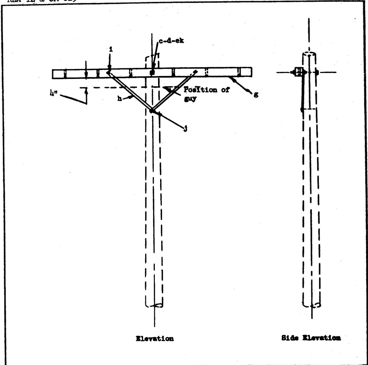
USED ON NON-JOINT OR JOINT TANGENT OR CORNER POLES FOR 4-INCH SPACED INSULATED OPEN WIRE USING T-21 AND T-22 STEEL BRACKET UNITS FOR WIRE ATTACHMENTS. LIMITATIONS: CORNERS 0 TO 35 DEGREES; 225 LBS. MAXIMUM VERTICAL LOAD PER CONDUCTOR; AND 10 PERCENT MAXIMUM DOWNWARD GRADE CHANGE. SEE FIGURES 9 AND 10 FOR WIRE ATTACHMENT METHODS.
