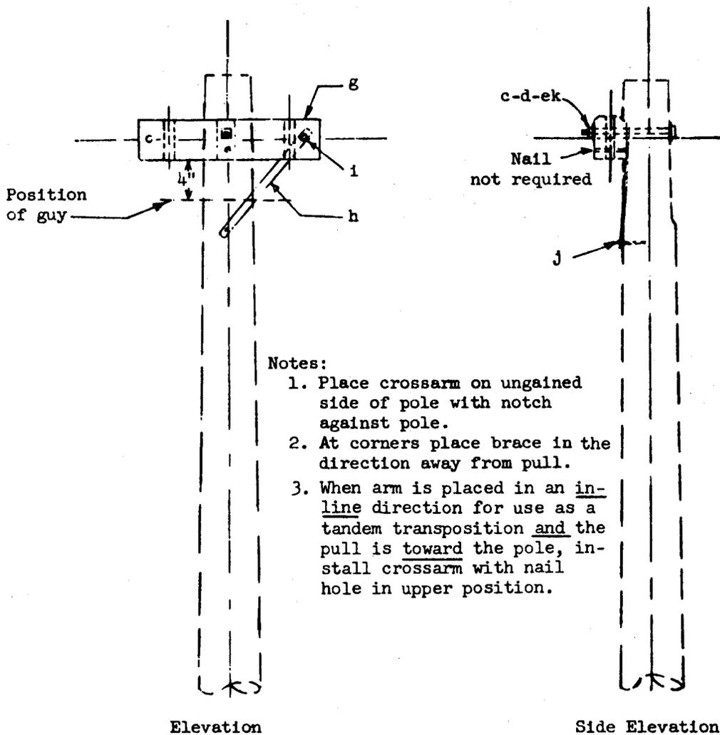
USED ON NON-JOINT CORNER POLES. LIMITATIONS: CORNERS 5 TO 35 DEGREES; 10 PERCENT MAXIMUM DOWNWARD GRADE CHANGE; 300 LBS. MAXIMUM VERTICAL LOAD PER CONDUCTOR.
