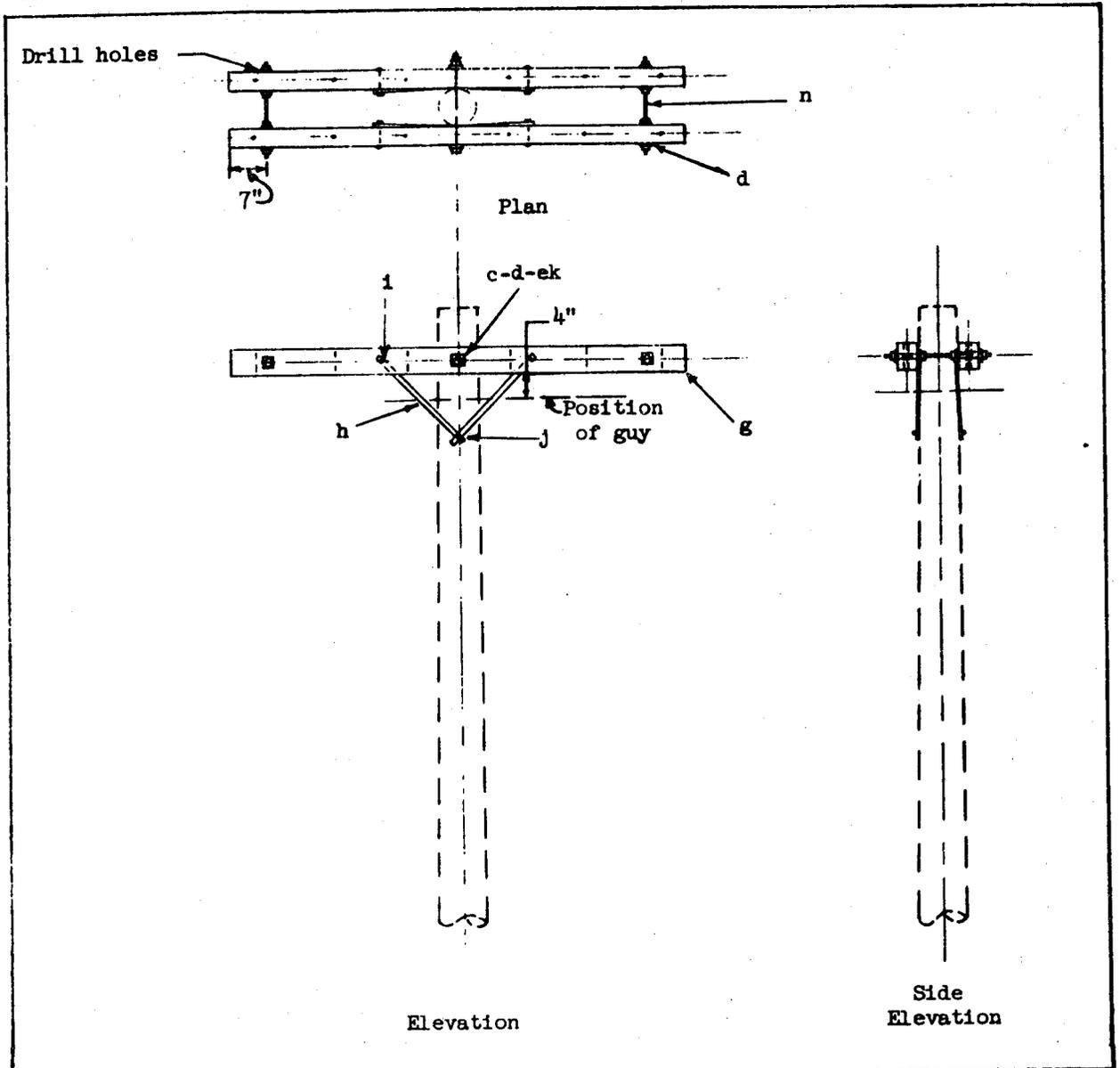
USED ON NON-JOINT POLES AT ALL RAILROAD AND RIVER CROSSINGS; ALSO AT CORNERS AND FOR DOWNWARD GRADE CHANGES, EXCEEDING 10 PERCENT. LIMITATIONS: CORNERS 35 TO 60 DEGREES; VERTICAL LOAD PER CONDUCTOR 225 TO 450 LBS. AND 25 PERCENT MAXIMUM DOWNWARD GRADE CHANGE.
