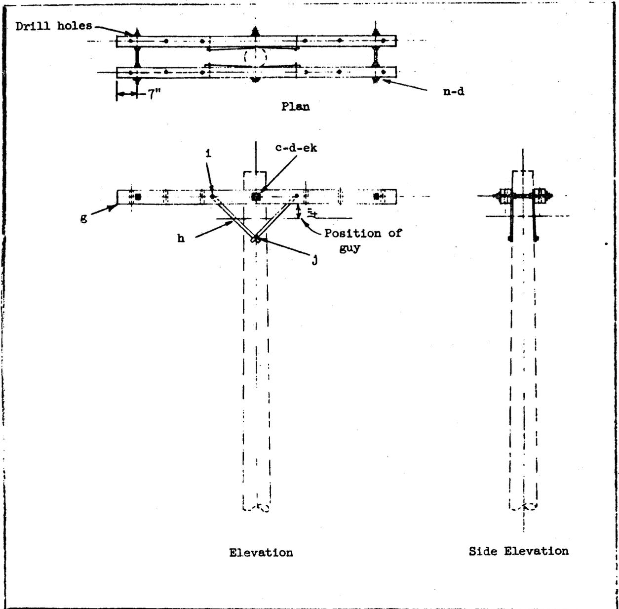
USED ON JOINT POLES IF DOUBLE ARMS ARE NECESSARY; ALSO ON JOINT LINES AT ALL RAILROAD AND RIVER CROSSINGS AND IS PERMISSIBLE ON NON-JOINT EXTENSIONS TO JOINT LINES; ALSO AT CORNERS AND FOR DOWNWARD GRADE CHANGES EXCEEDING TEN PERCENT. LIMITATIONS: CORNERS 35 TO 60 DEGREES; VERTICAL LOAD PER CONDUCTOR 225 TO 450 POUNDS, AND 25 PERCENT MAXIMUM DOWNWARD GRADE CHANGE.
