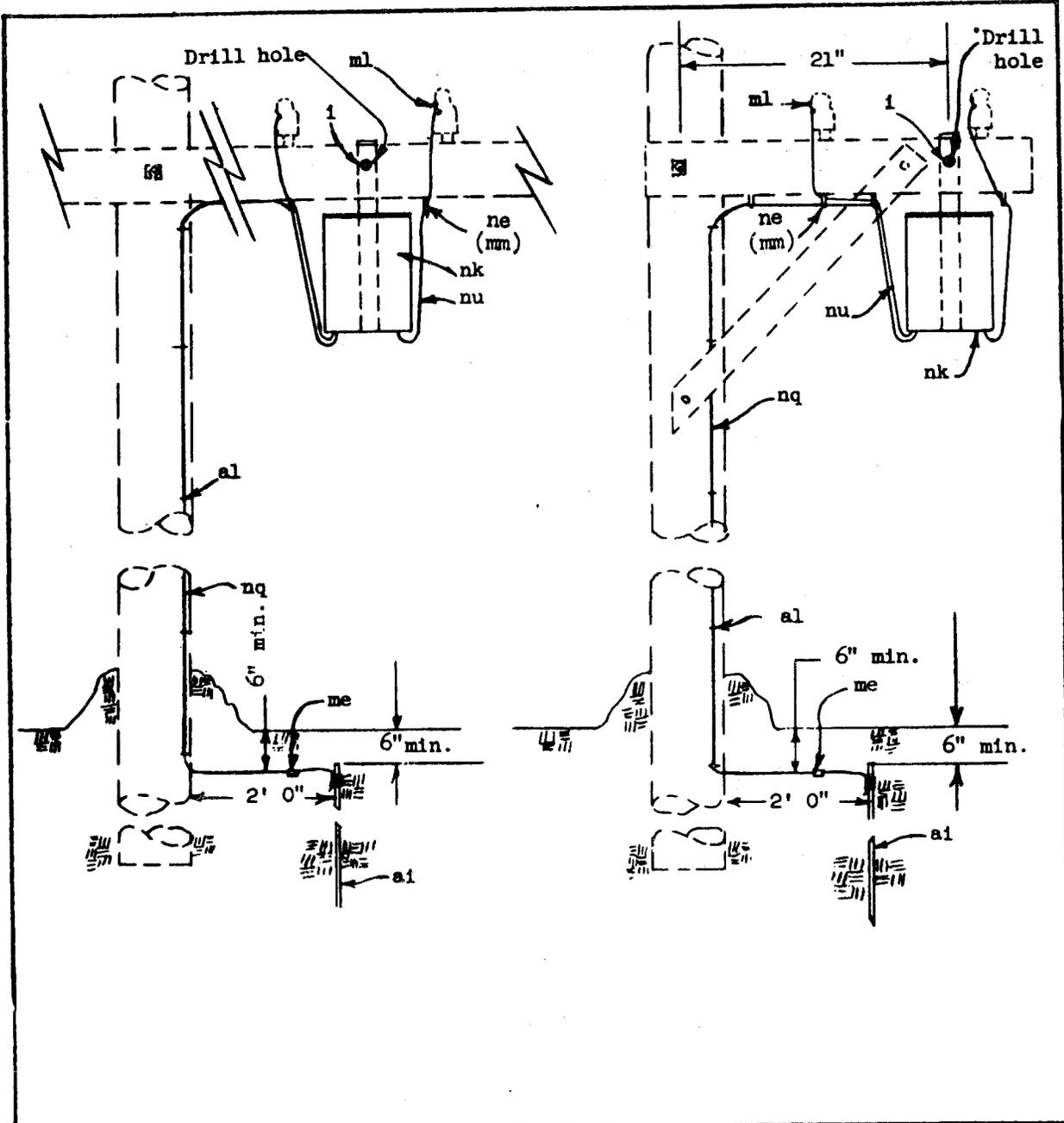
USED TO PROVIDE DRAINAGE PROTECTION ON ONE JOINT USE OPEN WIRE. CIRCUIT ON POLES CARRYING OTHER THAN MGN TYPE POWER CIRCUITS. SEE REA TE & CM-820, "OPEN WIRE CIRCUIT PROTECTION," FOR APPLICATIONS.
