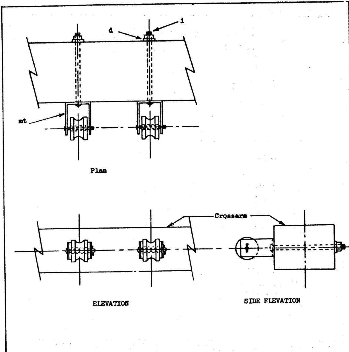
USED FOR DEADENDING CIRCUITS ON A CROSSARM WHERE THE WIRE PULL ON EACH INSULATOR KNOB WILL NOT EXCEED 1500 LBS. SEE GUIDE DRAWINGS 165 AND 165-1, ALSO PBI-6 AND PBI-7.
