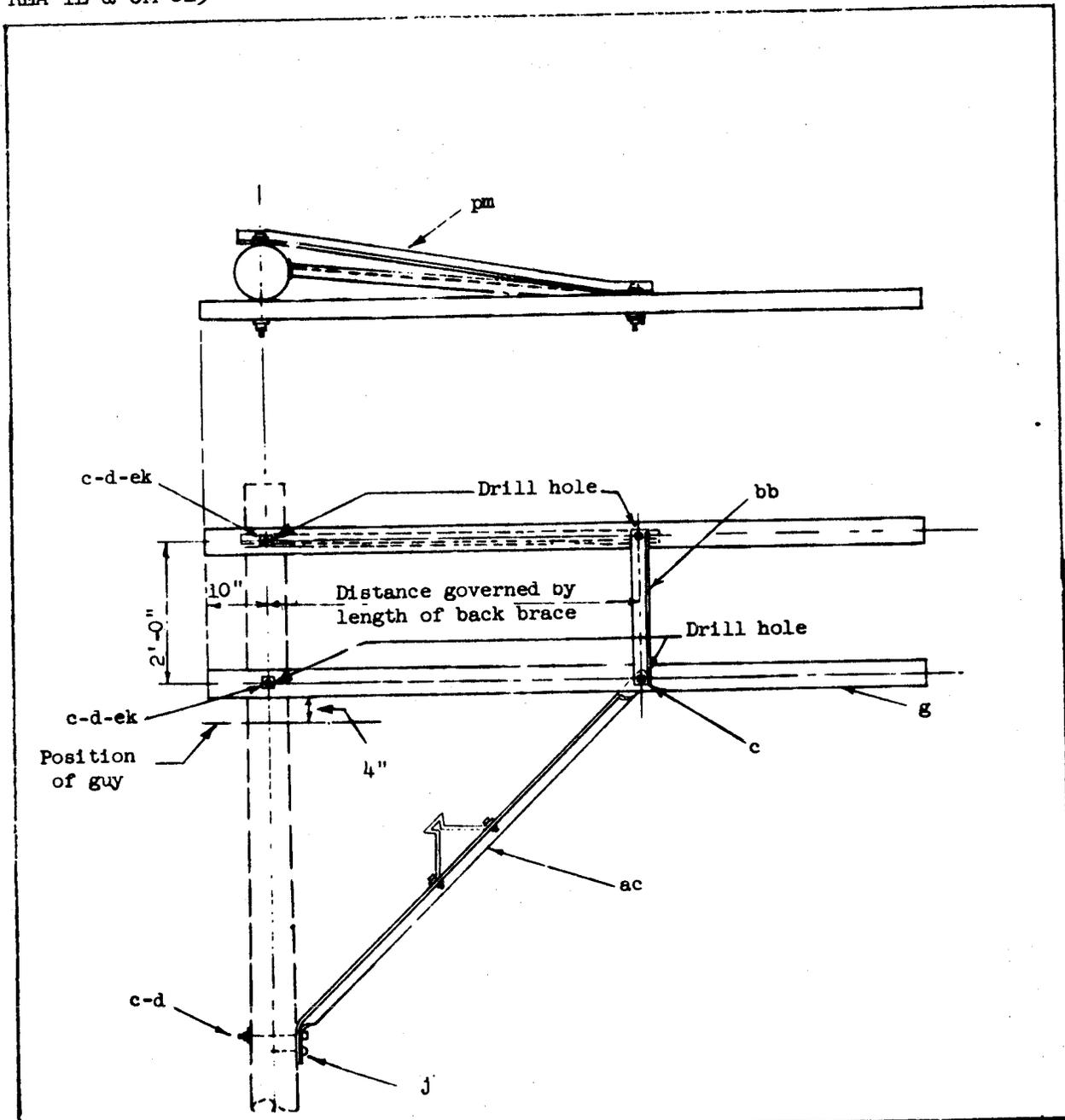
USED ON TWO CROSSARM NON-JOINT POLES TO AVOID TREES OR OTHER OBSTRUCTIONS. LIMITATIONS: MAXIMUM CORNER FIVE DEGREES WITHOUT GUY; 225 POUNDS MAXIMUM VERTICAL LOAD PER CONDUCTOR; TEN PERCENT MAXIMUM DOWNWARD GRADE CHANGE. REQUIRES POLE ONE CLASS LARGER THAN OTHERS IN NON-JOINT LINES.
