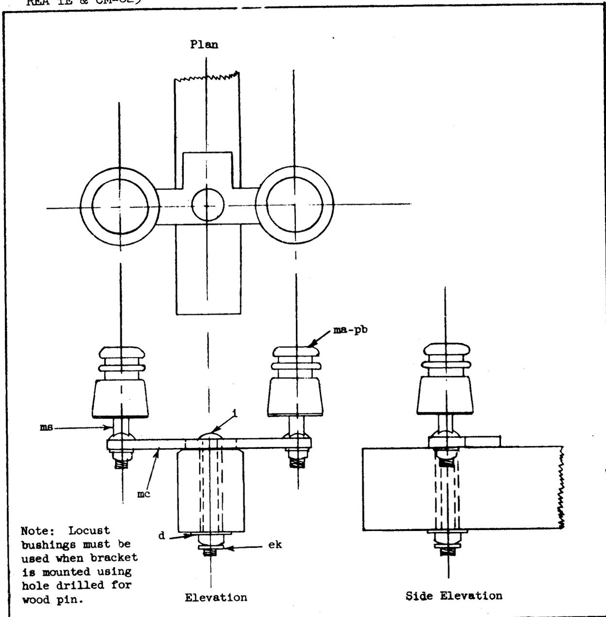
Note: Locust bushings must be used when bracket is mounted using hole drilled for wood pin.
