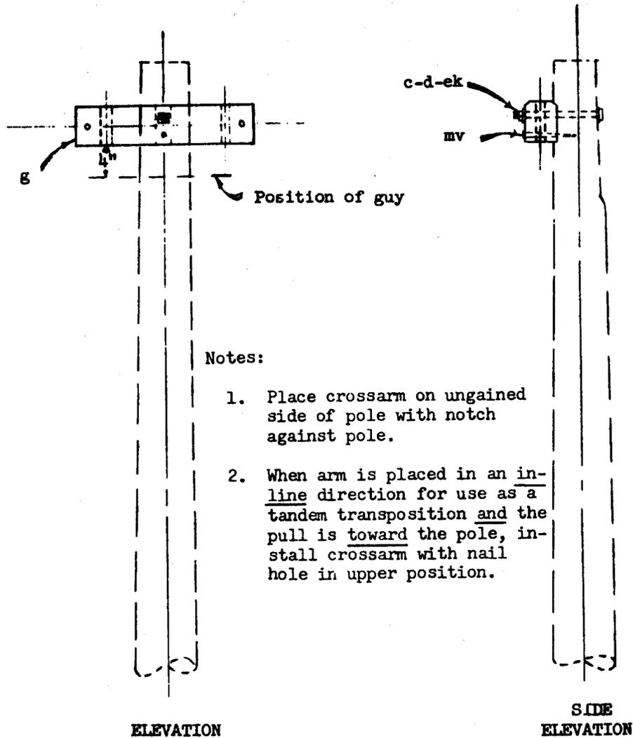
USED ON NON-JOINT POLES: ALSO AS A TANDEM TRANSPOSITION WITH THE CROSSARM PLACED IN LINE WITH THE WIRES AND USING A T-3 PIN AND INSULATOR UNIT. LIMITATIONS: CORNERS NOT TO EXCEED 5 DEGREES: 300 LBS. MAXIMUM VERTICAL LOAD PER CONDUCTOR: AND 10 PERCENT MAXIMUM DOWNWARD GRADE CHANGE. SEE GUIDE DRAWINGS 121-1 AND 121-4 FOR PLACEMENT OF THIS CROSSARM.
