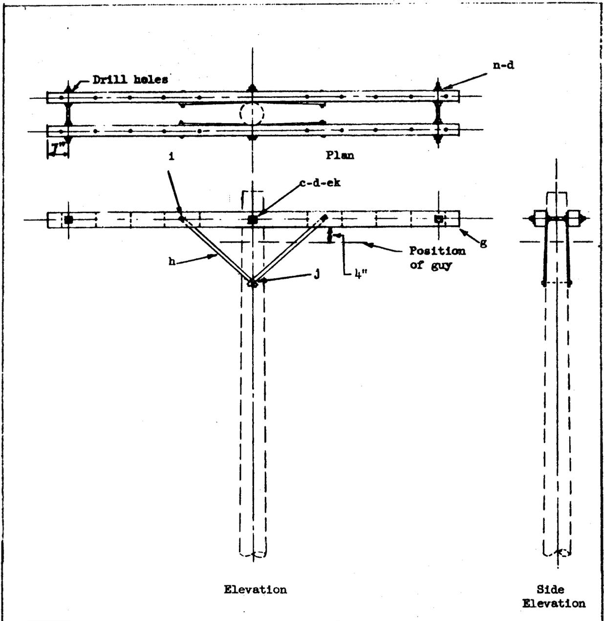
USED ON JOINT POLE IF DOUBLE ARMS ARE NECESSARY, ALSO ON JOINT LINES AT ALL RAILROAD AND RIVER CROSSINGS AND IS PERMISSIBLE ON NON-JOINT EXTENSIONS TO JOINT LINES; ALSO AT CORNERS AND FOR DOWNWARD GRADE CHANGES EXCEEDING TEN PERCENT. LIMITATIONS: CORNERS 35 TO 60 DEGREES; VERTICAL LOAD PER CONDUCTOR 225 TO 450 POUNDS, AND 25 PERCENT MAXIMUM DOWNWARD GRADE CHANGE.
