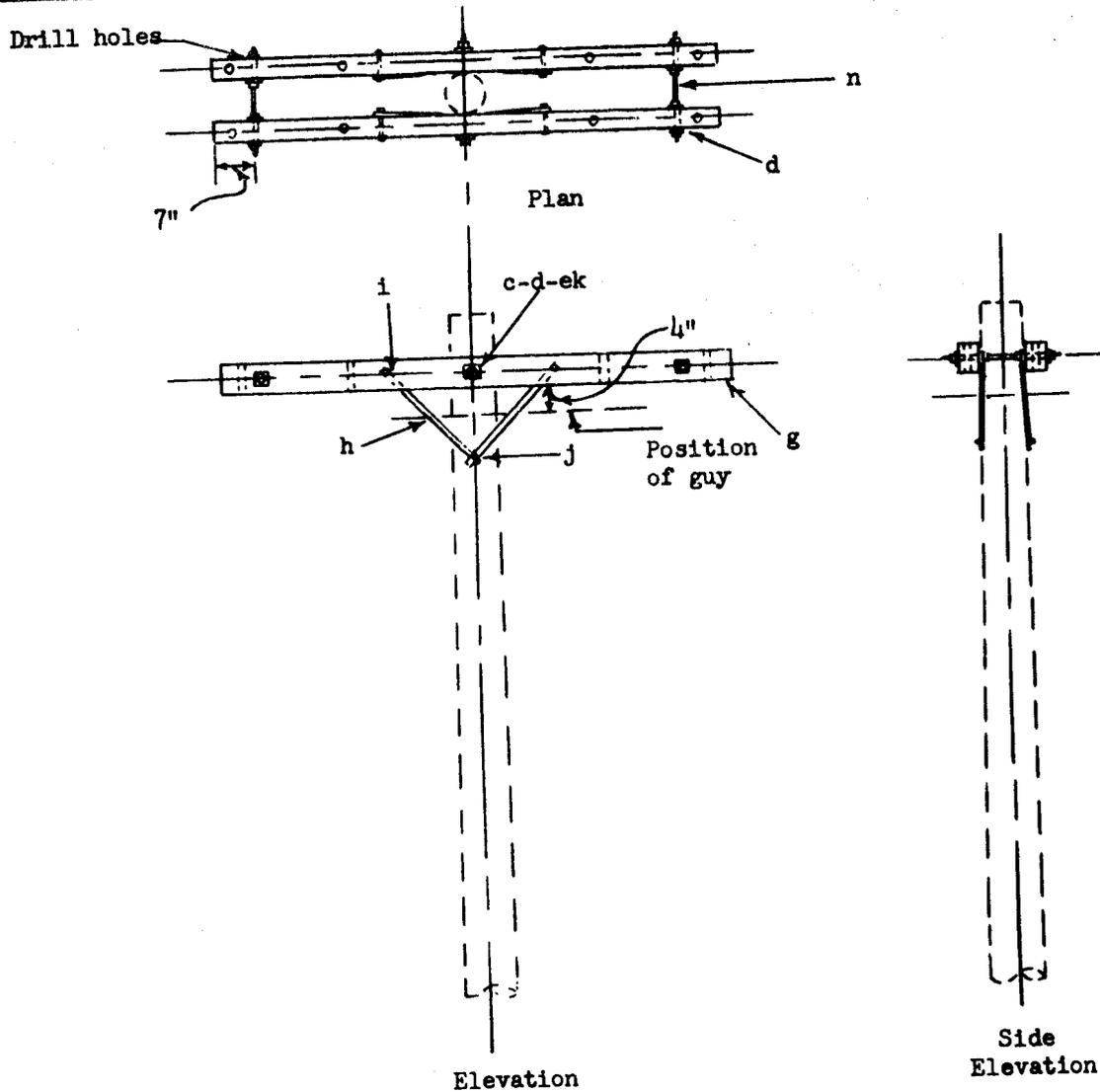
USED ON NON-JOINT OR JOINT TANGENT OR CORNER POLES FOR 4-INCH SPACED INSULATED OPEN WIRE USING T-21 STEEL BRACKET UNITS FOR WIRE ATTACHMENTS; AT ALL RAILROAD AND RIVER CROSSINGS IN SUCH LINES: AND AT DOWNWARD GRADE CHANGES EXCEEDING 10 PERCENT. LIMITATIONS: CORNERS 35 TO 60 DEGREES; VERTICAL LOAD PER CONDUCTOR 450 LBS.; AND 25 PERCENT MAXIMUM DOWNWARD GRADE CHANGE. SEE FIGURE 11 FOR WIRE ATTACHMENT METHODS.
