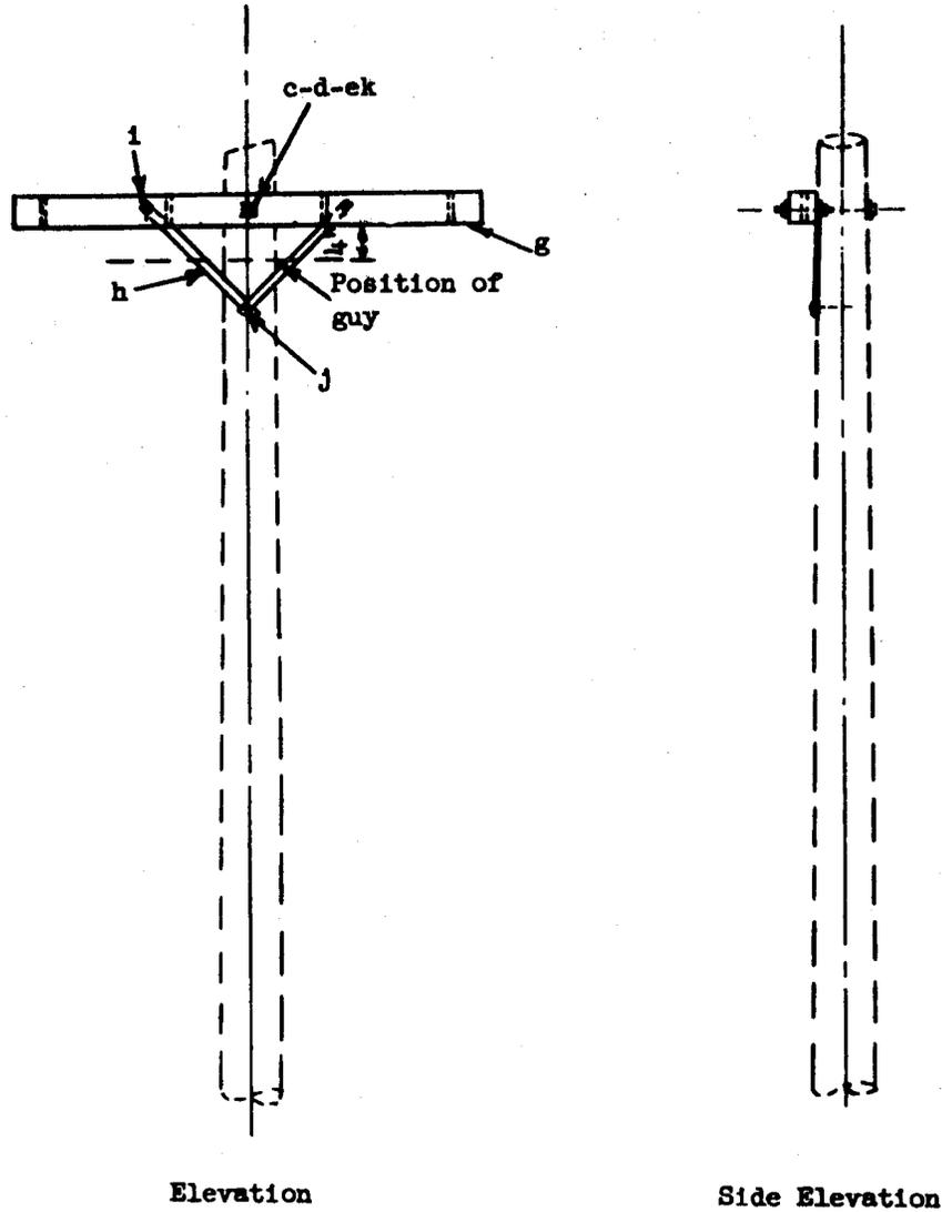
USED ON NON-JOINT OR JOINT TANGENT OR CORNER POLES FOR 4-INCH SPACED INSULATED OPEN WIRE USING T-21 OR T-22 STEEL BRACKET UNITS FOR WIRE ATTACHMENTS. LIMITATIONS: CORNERS 0 TO 35 DEGREES; 225 LBS. MAXIMUM VERTICAL LOAD PER CONDUCTOR; AND 10 PERCENT MAXIMUM DOWNWARD GRADE CHANGE. SEE FIGURES 9 AND 10 FOR WIRE ATTACHMENT METHODS.
