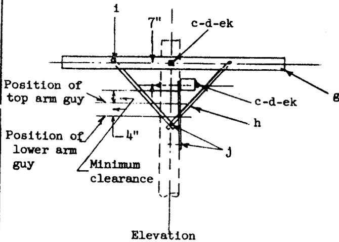
WHERE ONE OF THE TWO SPANS HAS AN UP-PULL PLACE ITS CIRCUITS ON UPPER CROSSARM. IF ONE HAS A DOWNPULL PLACE ITS CIRCUITS ON LOWER ARM. IF BOTH SPANS PULL UP OR DOWN ADJUST SEPARATION OF CROSSARMS TO GIVE INCREASED SEPARATION BETWEEN THE WIRES IN THE TWO SPANS.
