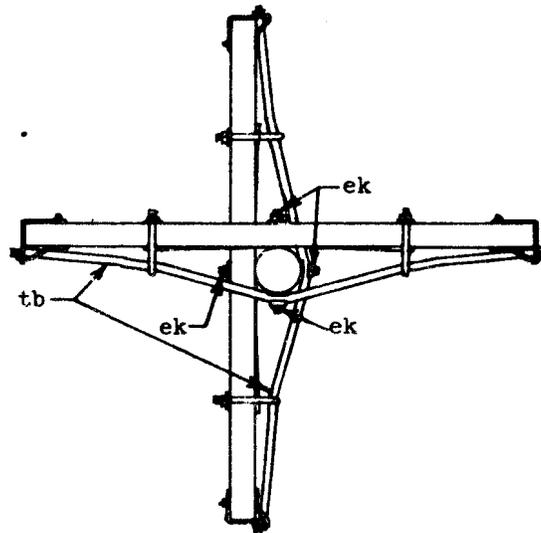
USED AS DEADENDS IN JOINT OR NON-JOINT CONSTRUCTION TRANSPOSED ACCORDING TO REA TE & CM-463, "REA-1 TRANSPOSITION SYSTEM."
