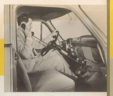
It provides communication between mobile units and any telephone reached by the Bell System, or between two mobile units.
