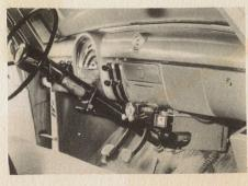
CONTROL UNIT — The small control unit is mounted in automotive equipment conveniently under the instrument panel. It is simple to operate, with no tuning required. The hand telephone fits snugly in the receptacle built into the control unit and automatically operates the switch hook—much the same as the "hook" on your home telephone.
