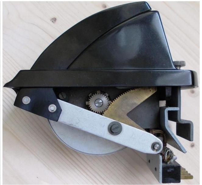
Part of the text belonging to exhibit 3-6-4B states that "... the insides [are] partially uncovered, so as to reveal some of the operating mechanism inside." This is incorrect, in that, since these dials were installed on switchboards, only the portion up to, and including, the finger stop, was visible. The rest of the dial was below the surface of the switchboard keyshelf, and required no further (dust) protection other than a round, aluminum case for the dial mechanism itself ...
