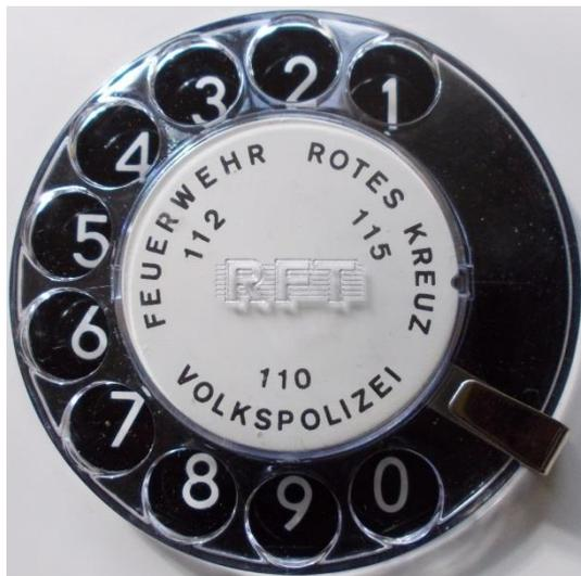
This is the mechanical dial of a GDR desk set ("Alpha Ferro") from the mid-1980s, approximately the same time the drop-in keypad was placed into service.
