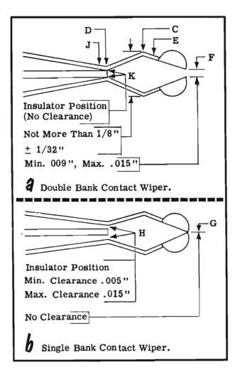
Figure 9. Wiper Tip and Insulator Clearance Requirements.
