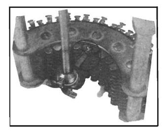
Figure 15. A Wiper Spring Assembly which is Bridging Between Bank Contacts 5 and 6. Level O.
