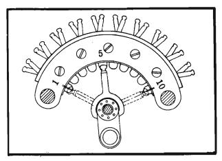
Figure 14. Rotary Centering is Checked on Contacts 1, 5, and 10 and Adjusted on Contact 5.
