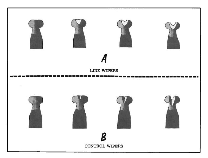
Figure 2. Examples of Wiper Tips That Are in Various Stages of Wear. (Note That Line Wiper Tip Wear is Distributed Over a Wider Tip Area Than Control Wiper Tip Wear.)
