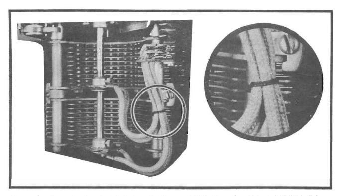
Figure 4. Example of a Switch that is Not Equipped With Wiper Cord Bracket, With the Wiper Cords Properly Tied.
