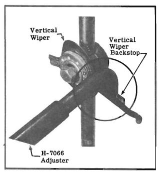
Figure 19. Method for Adjusting Vertical Wiper Backstop is Shown in Circle.
