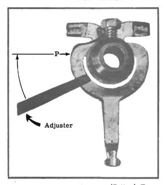
Figure 12. Remove Tension (Follow) From Line and Control Wiper Spring by Working Adjuster to Point P.
