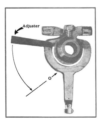
Figure 11. An Adjuster is being Used to Add Tension (Follow) to Line and Control Wiper Springs.
