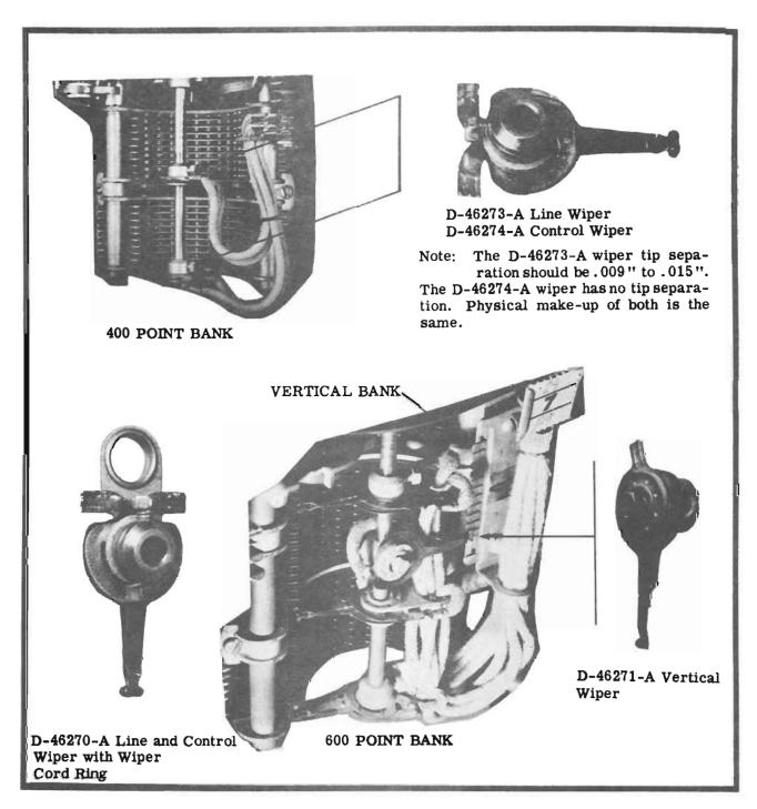
Figure 1. Above are the Wiper Assemblies Referred to in this Practice and Examples Showing Where Each Type is Used. (The 400 Point Bank, Shown, Takes Two D-46273-A Line Wipers. The 300 Point Bank, Not Shown, Takes One D-46273-A Line Wiper and One D-46274-A Control Wiper.)
