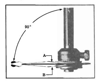
Figure 7. Properly Formed Wiper Springs are Shown Above.
