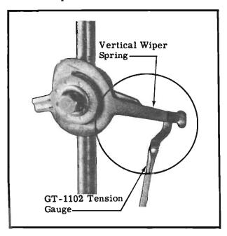
Figure 21. Tension Gauge is Being Used for Checking Vertical Wiper Spring Tension.
