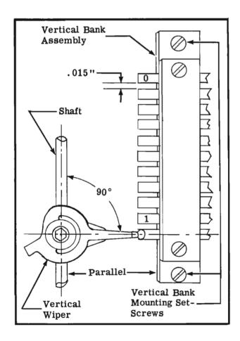
Figure 18. The Vertical Wiper Assembly and Vertical Bank is Shown With Related Requirements.
