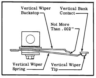
Figure 20. Above is a Side View of the Vertical Wiper and Backstop Requirements.
