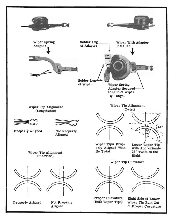
Figure 3. The Above Are Wiper Spring Assemblies, Wiper Spring Adapters, and Examples of Alignment.
