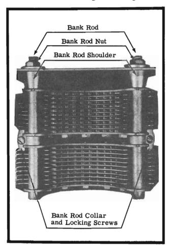
Figure 17. A 400 Point Bank with Arrows Indicating Bank Rods, Bank Rod Nuts, Bank Rod Shoulders, Bank Rod Collars and Locking Screws.
