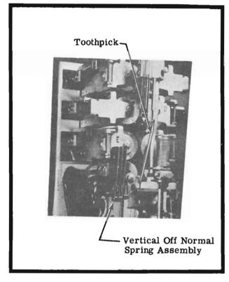
Figure 5. One Method for Opening the Release Circuit of a Strowger Two Motion Switch is by the Use of a Toothpick.
