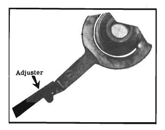
Figure 16. A Wiper Tip Ear being bent by an Adjuster.
