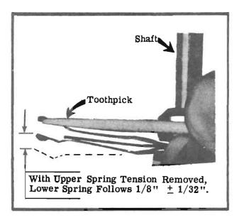
Figure 10. A Toothpick can be used for Checking Wiper Spring Tension (Follow) and Requirements. (Procedure Shown is Reversed When Checking Upper Wiper Spring Tension.)
