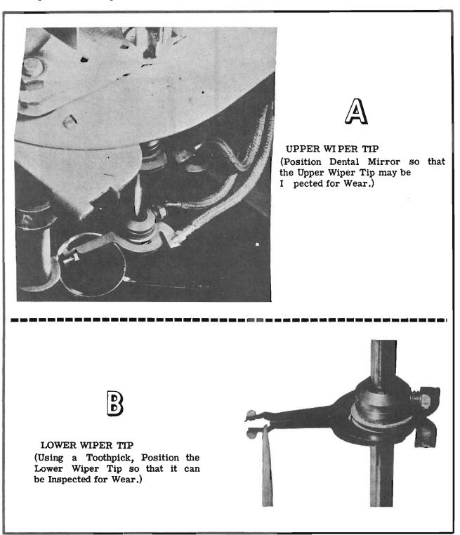
Figure 6. The Above Method is Used When Inspecting Upper and Lower Wiper Tips for Wear.
