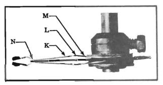
Figure 8. Properly Spaced Wiper Springs are Shown Above.
