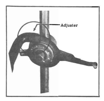
Figure 22. Spring Adjuster is Being Used to Adjust Tension of Vertical Wiper Spring.
