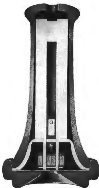
Cross Section, No. 144 Receiver
