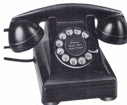
BELL IN BASE OF COMBINATION HANDSET
