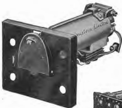
No. 30C Supervisory Signal Shutter Restored
