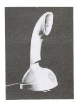
2.02 The Ericofon is a light-weight one-piece stand type telephone with receiver in the top end, transmitter in the top of the base and dial in the bottom end of the base as illustrated on Page 3. In its normal standing position it resembles an ornamental vase that appeals to the eye. It weighs 15 ounces.
