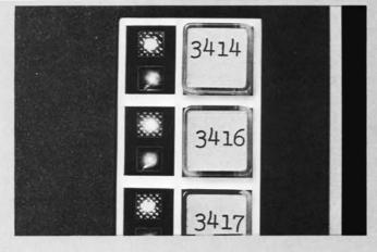
Light-emitting diodes give a continuous reading of each button on the telephone. RED indicates the line the customer has selected, and GREEN tells the status of each line—busy, idle, ringing, or on hold. The buttons, which do not lock when pressed, access features or serve as line pickups.
