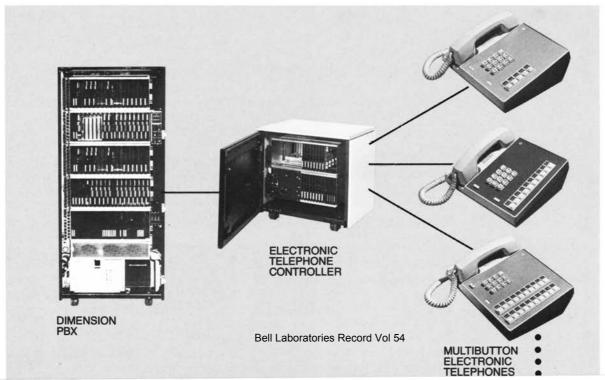
ory. This memory contains data reflecting the status of the buttons, lamps, switchhooks, and ringers in the electronic telephones.
