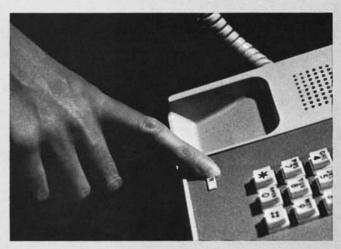
The Recall button eliminates the need to flash the switchhook to access special features.
