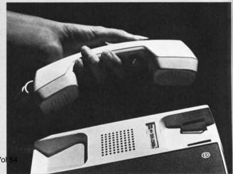
The MAAP in the DIMENSION PBX is used to change telephone features and line pickup assignments and to liagnose system problems.
