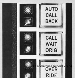
Custom-calling feature buttons replace dial codes. For example, after receiving a busy signal, a DCTS customer has several options: press Automatic Callback and when the line is free be called back automatically; press Call Waiting-Originating to send a special tone that lets the busy extension know a call is waiting; or press Executive Override to talk to the called party immediately.
