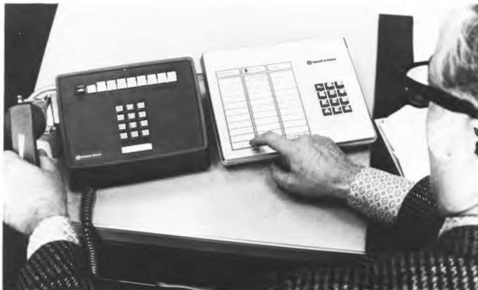
Handy helper. The standard Touch-A-Matic telephone furnishes from one to five telephone lines. Whenever more lines are needed, the convenience of automatic dialing may be provided by the Touch-A-Matic dialer (right), used in conjunction with a Call Director telephone, a Cor Key set, or a 10- or 20-button key telephone.
