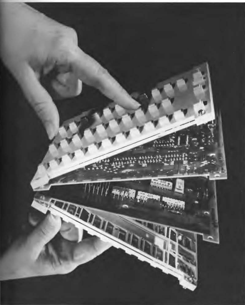
Mirror image. The memory unit of the Touch-A-Matic telephone consists of both a button and contact spring assembly (top) and a printed wiring board (PWB) assembly (just underneath), both shown suspended over a mirror so that the undersides of the assemblies can be seen. When a user touches a memory button, a contact spring beneath the button makes contact with a gold-plated pad on the top of the epoxy glass PWB. The pads are connected directly to the silicon integrated memory circuits and other electronic components on the underside of the PWB. The circuits connect to the remainder of the set via the connector pins, which are on the component side of the PWB.
