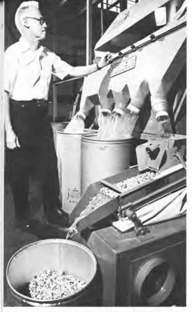
Final sorting. Heavy contaminants fall into the left bin and partially separated pellets that must be resorted into the center bin. Special equipment (right foreground) removes any remaining metallic bits from the pellets falling into the recycling bin.
