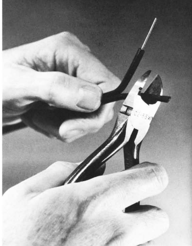
places and does not kink. The new wire's 10 percent lower cost means large savings for the Operating Companies. PVC-insulated drop wire can be stripped with a pair of ordinary diagonal pliers, shown at right. The old wire requires a special stripping tool.
