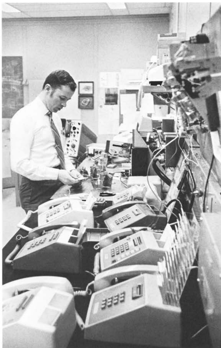
Co-author Dan Miller runs a test on a TOUCH-TONE® credit-card dialer mechanism in a room containing several assembled units at the Indianapolis, Indiana, location of Bell Laboratories.
