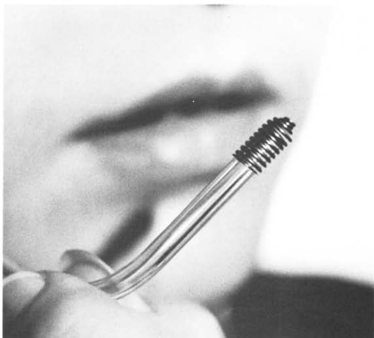
The speech-tube assembly comprises a metal tube with a ball joint and a plastic tube, which slides along the metal tube. The end of the plastic tube contains a porous metal disc for absorbing acoustic resonance and a wire tip that softens harsh sounds.
