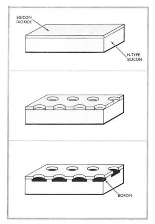
Major processing steps (sequentially top to bottom) in the fabrication of the diode array. It starts as a silicon wafer several thousandths of an inch thick. An oxide layer about 25 millionths of an inch thick is then grown on the surface of the silicon. Photo-lithographic techniques are used to generate an array of holes in the oxide. Boron is diffused into the silicon through the holes forming the p-type islands. In this step the remaining oxide serves as a diffusion mask.
