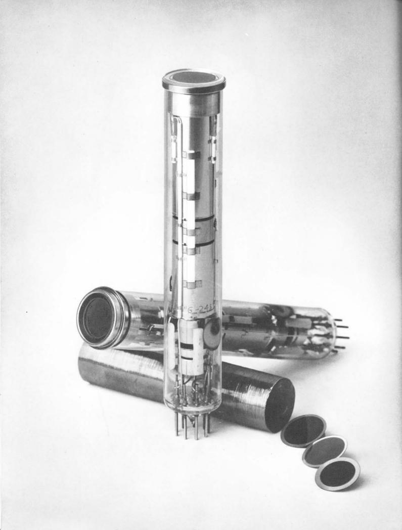
A new camera tube for the PICTUREPHONE set uses an integrated silicon photo-diode array combined with conventional electron beam scanning. The result is a vidicontype of camera tube which is far more sensitive and reliable than any now being used.
