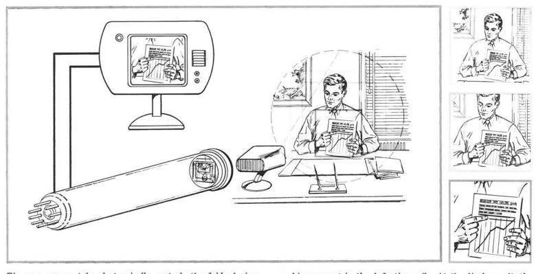
The new camera tube electronically controls the field of view of the displayed image by changing the size and position of the scanned area on the target. The camera lens produces a fixed-size image. The displayed image is defined by the raster which can be varied by varying the beam accelerating voltage
