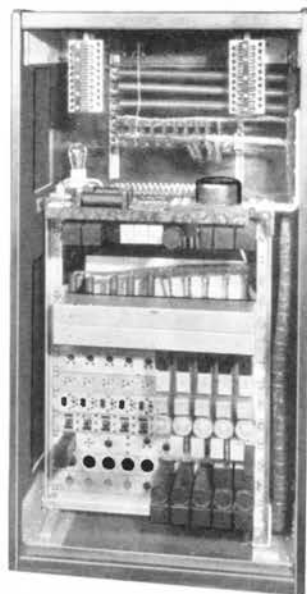
Fig. 3—Rear view of 551-A with gate closed showing relays mounted on outer side
